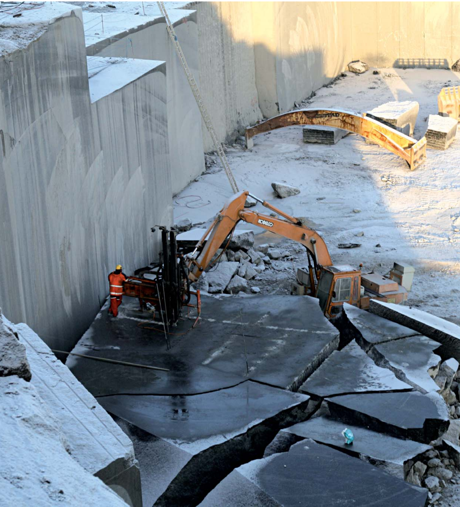
Production of larvikite blocks at the Lundh Labrador AS quarry at Klaastad. Photo: Peer-Richard Neeb.
