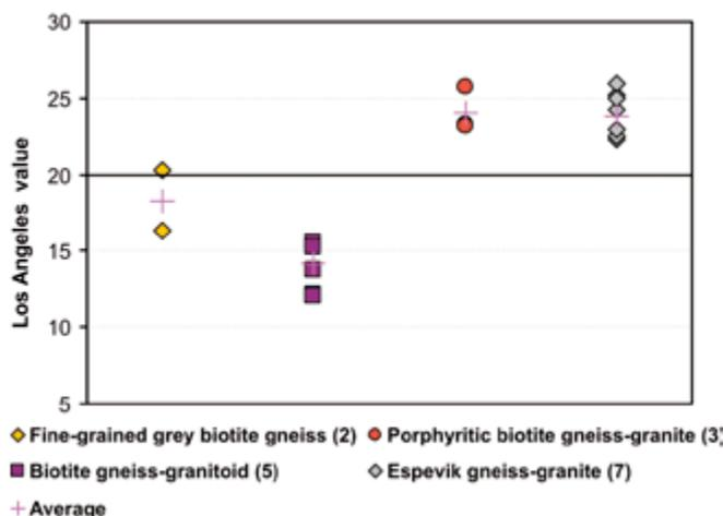
Figure 4. Variation in the Los Angeles value for different rock types (Marker and Erichsen 2002).
