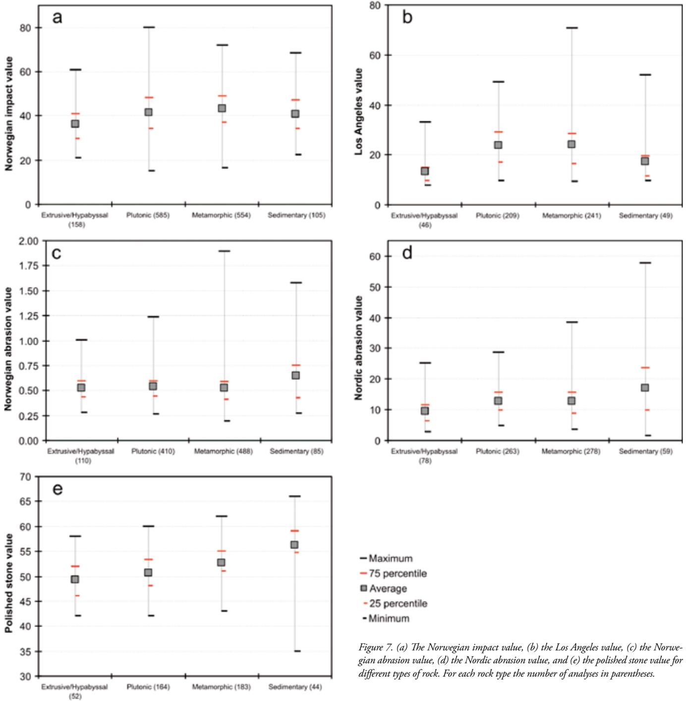
Figure 7. (a) The Norwegian impact value, (b) the Los Angeles value, (c) the Norwegian abrasion value, (d) the Nordic abrasion value, and (e) the polished stone value for different types of rock. For each rock type the number of analyses in parentheses.
