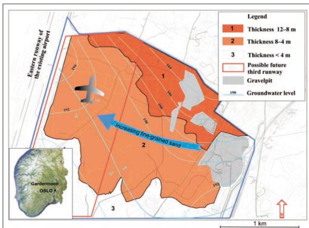
Figure 1. Variation in thickness in the investigated part of the Gardermoen sand and gravel deposit.
