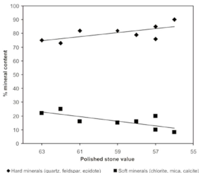
Figure 14. The variation in the polished stone value for Devonian sandstones depending on the mineral content.
