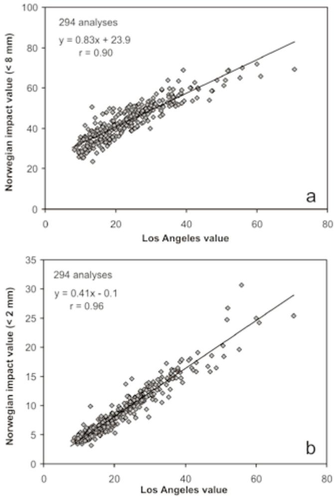
Figure 6. Los Angeles values versus Norwegian impact value (a) < 8 mm, (b) < 2 mm. Analyses from NGU's Database for hard-rock aggregates.
