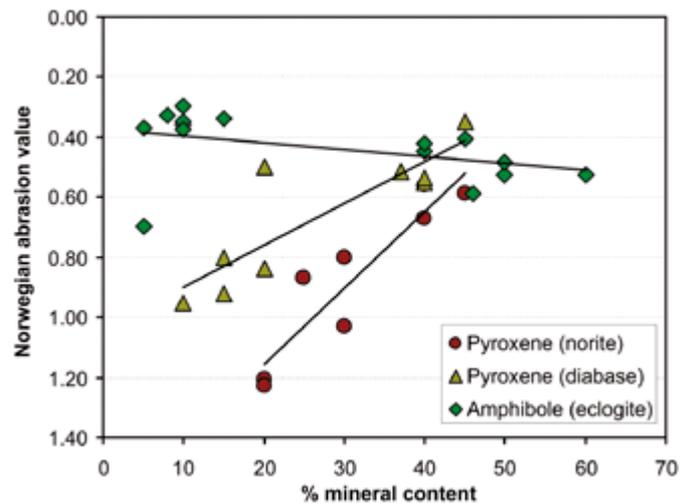
Figure 12. Variation in the Norwegian abrasion value depending on the mineral content for different rock types.
