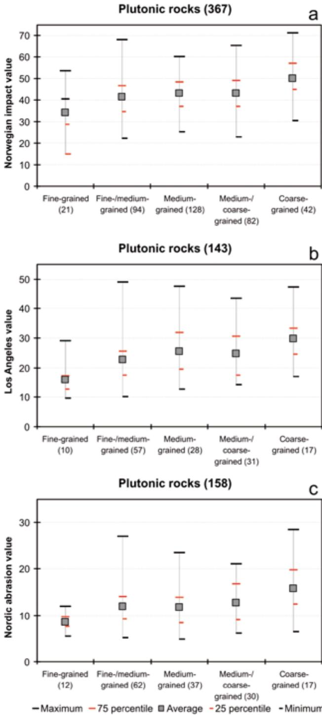
Figure 9. Variation in (a) the Norwegian impact value, (b) the Los Angeles value, and (c) the Nordic abrasion value with grain size for plutonic rocks. Number of analyses in parentheses.
