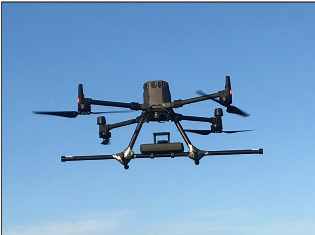
Figure 3: DJI M300 shortly before landing after a flight over the Fen area. The vector magnetometer is installed on the horizontal bar between the two legs forming the landing gear.
