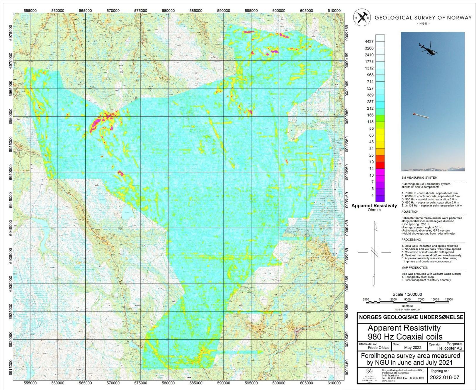
Figure 11: Apparent resistivity. Frequency 980 Hz, Coaxial coils
