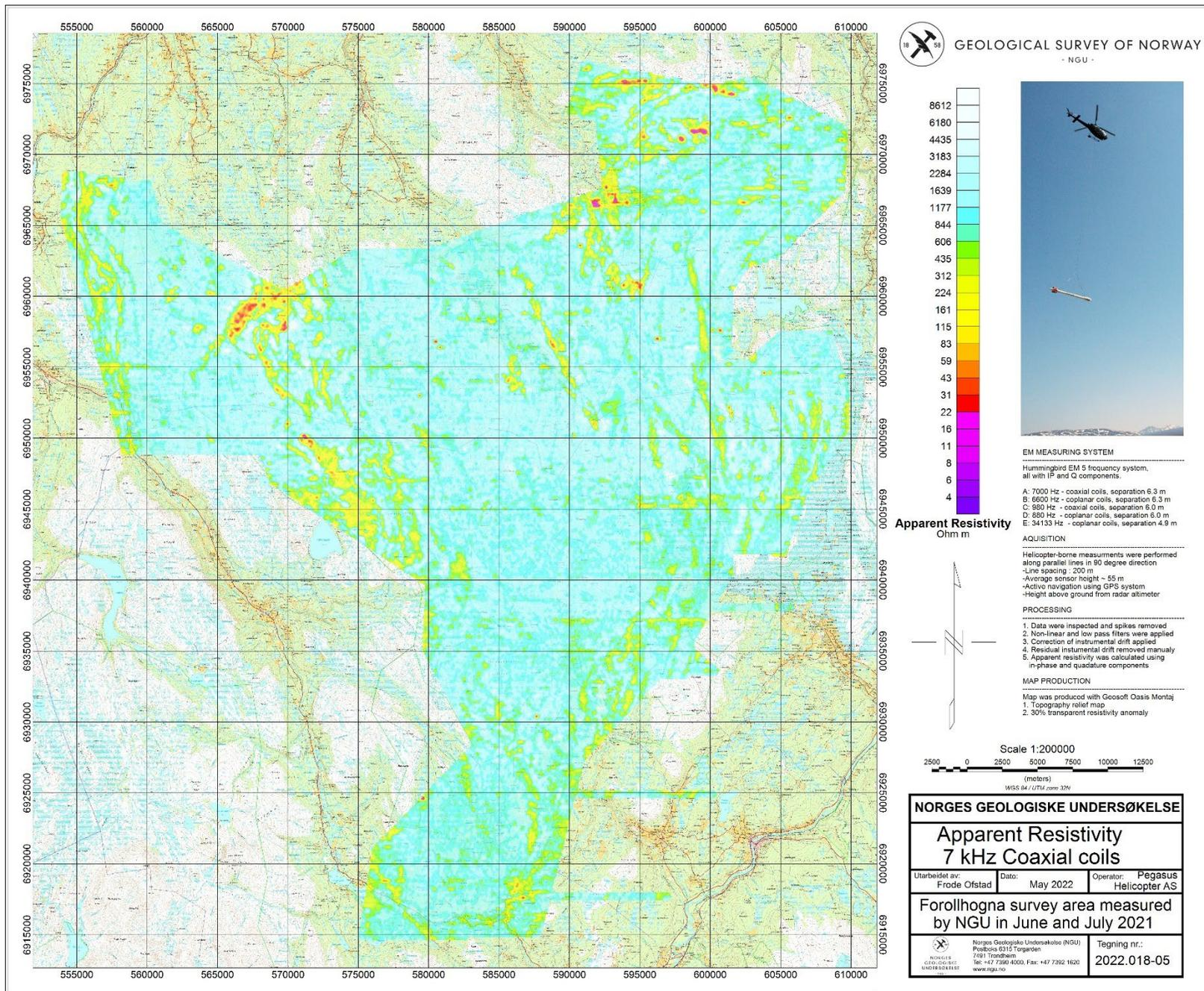
Figure 9: Apparent resistivity. Frequency 7001 Hz, Coaxial coils
