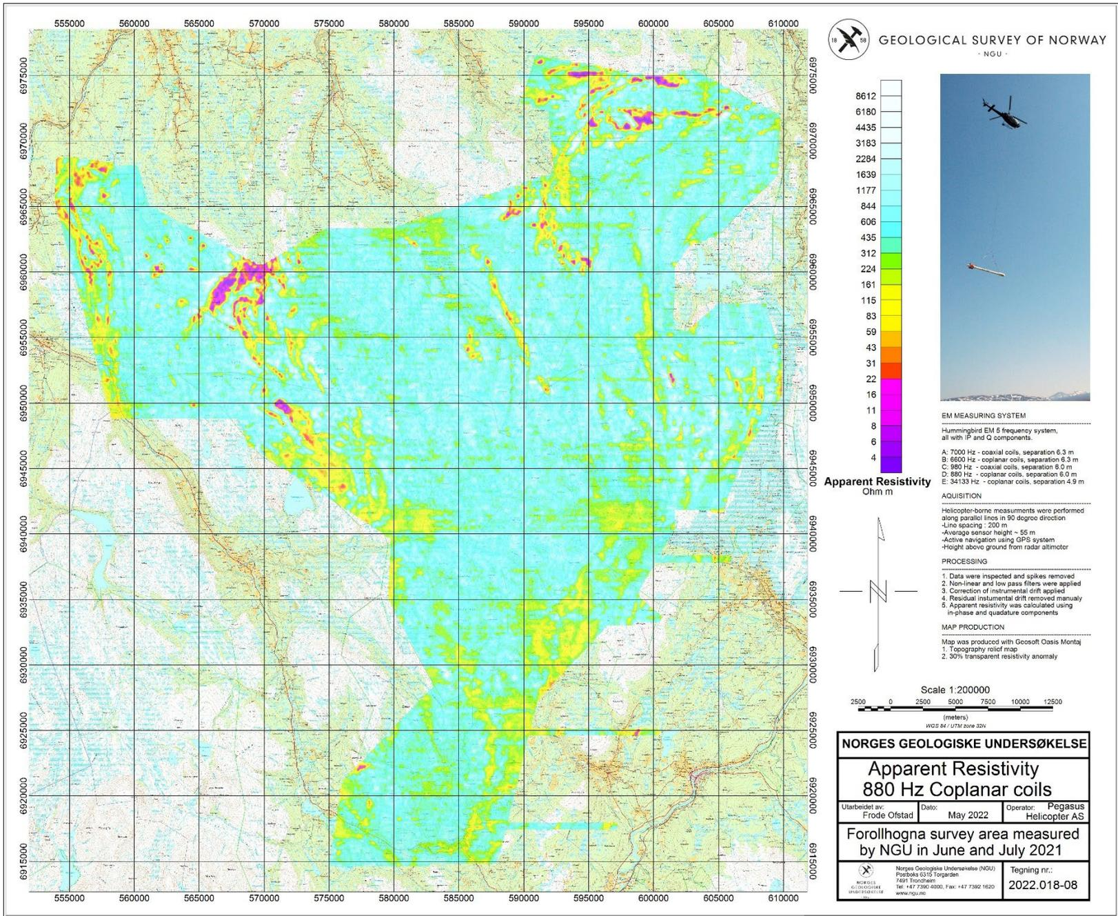
Figure 12: Apparent resistivity. Frequency 880 Hz, Coplanar coils
