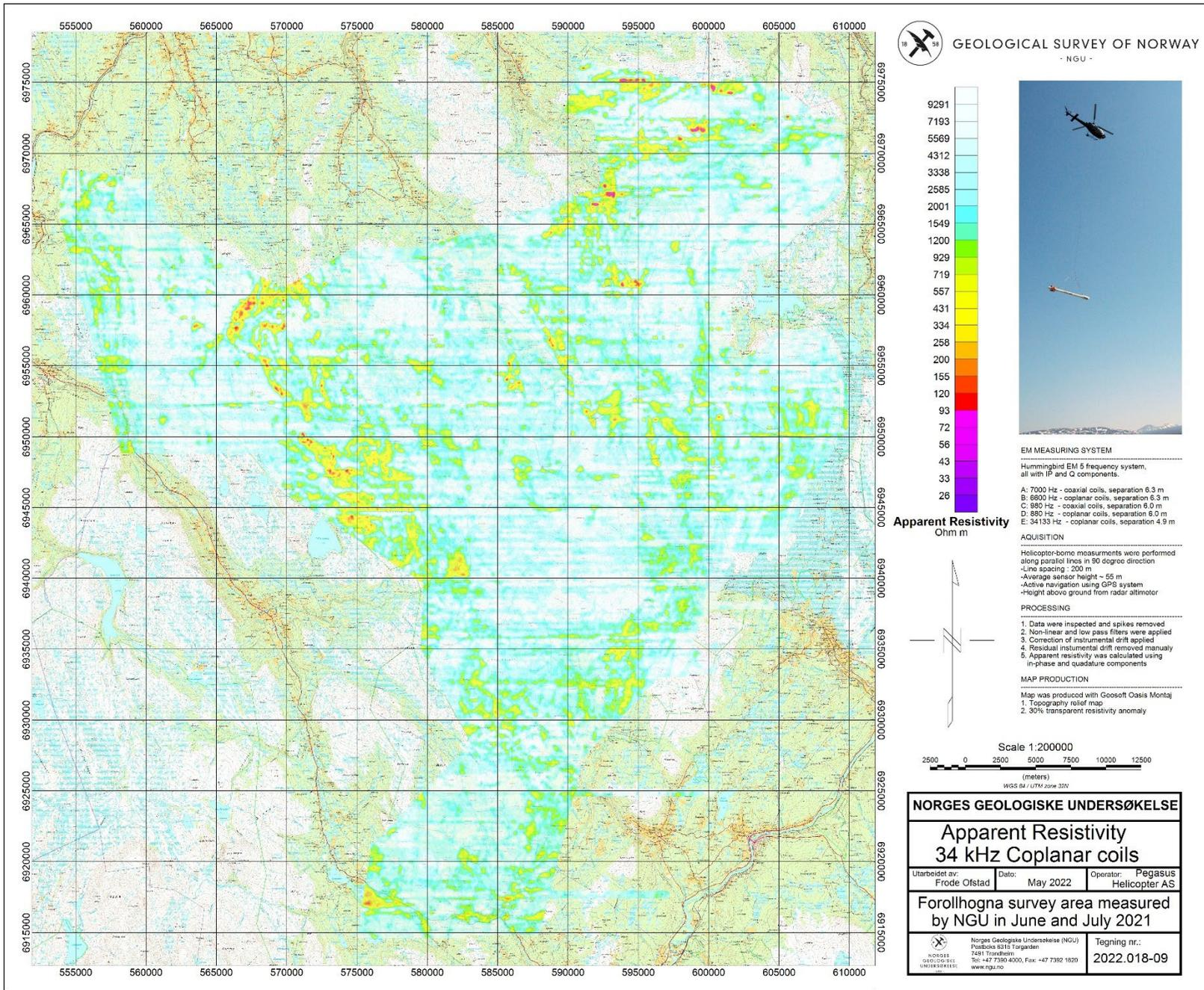
Figure 13: Apparent resistivity. Frequency 34133 Hz, Coplanar coils
