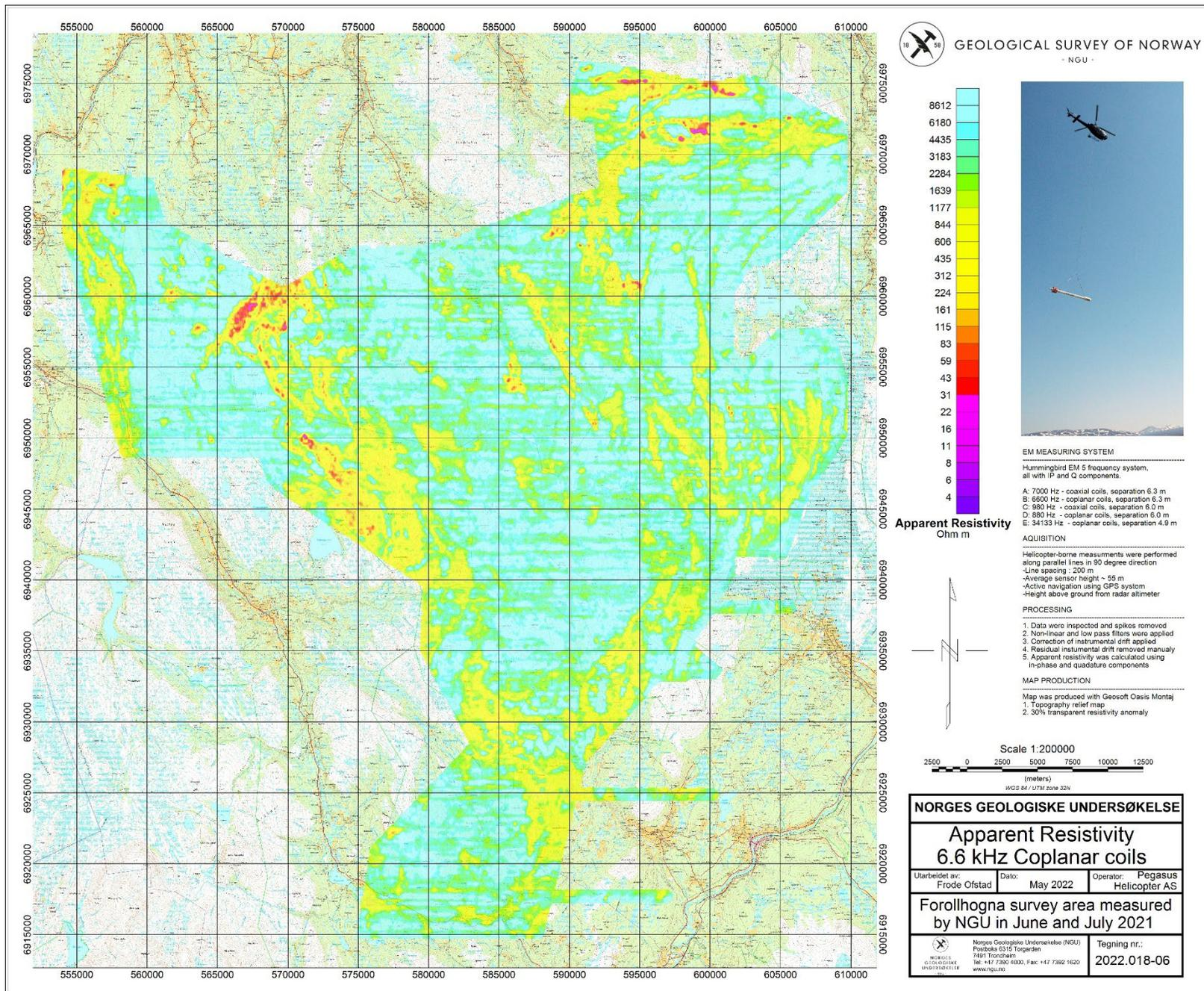
Figure 10: Apparent resistivity. Frequency 6606 Hz, Coplanar coils
