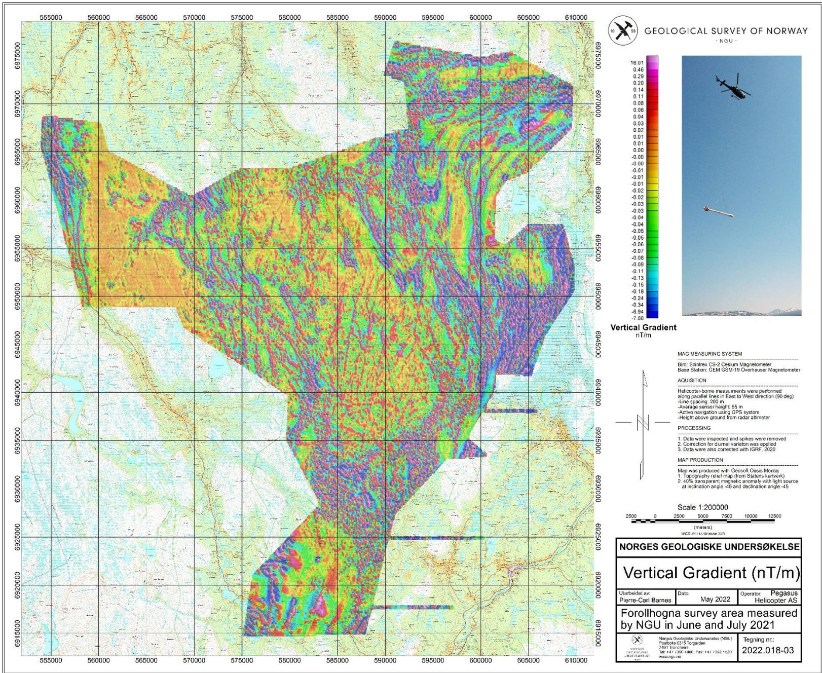
Figure 7: Magnetic Vertical Gradient
