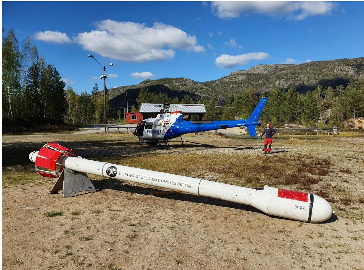
Figure 2: Pegasus helicopter, pilot, and NGU Hummingbird EM system
