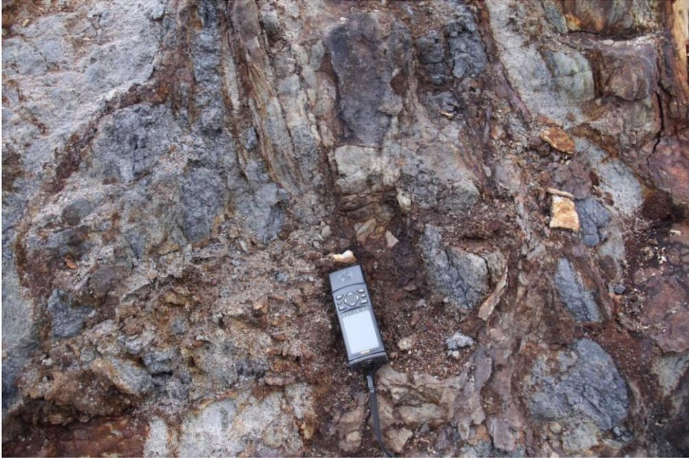
**Figure 8.8: Graphite location in road-cut near Langstrand (UTM WGS84 500625 – 7634012). A sample from this location (hg21-16) showed 25.6 % TC and 4.0 % TS.**
