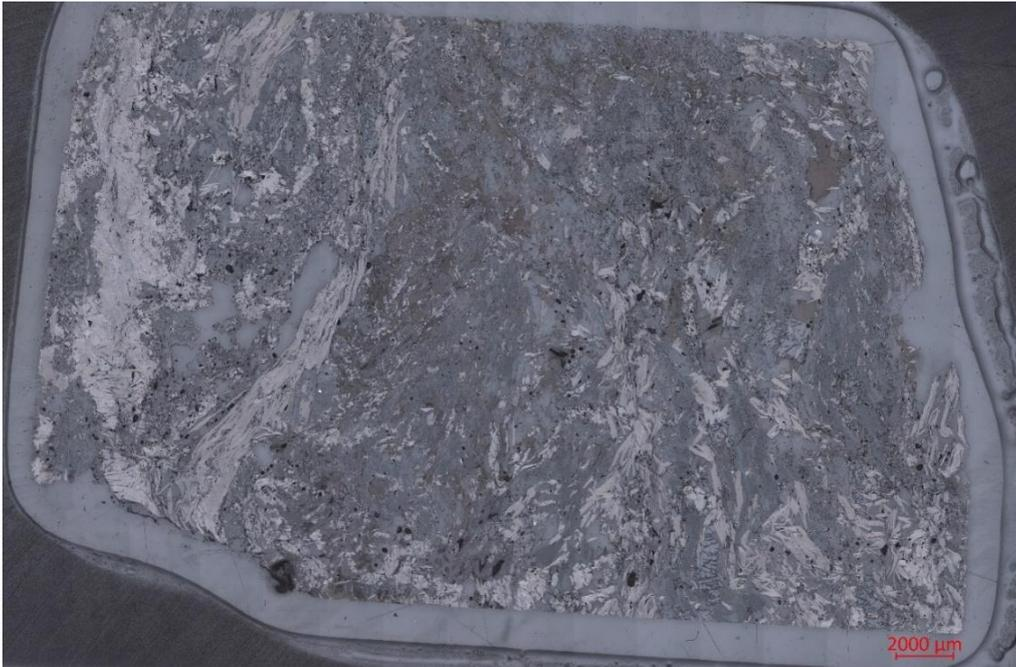
Figure 10.2: Graphite observed in reflected light, displaying variations in the distribution and grain size of the graphite flakes (thin section JK-2617-1, Sommarhus. TC = 24,7 %).
