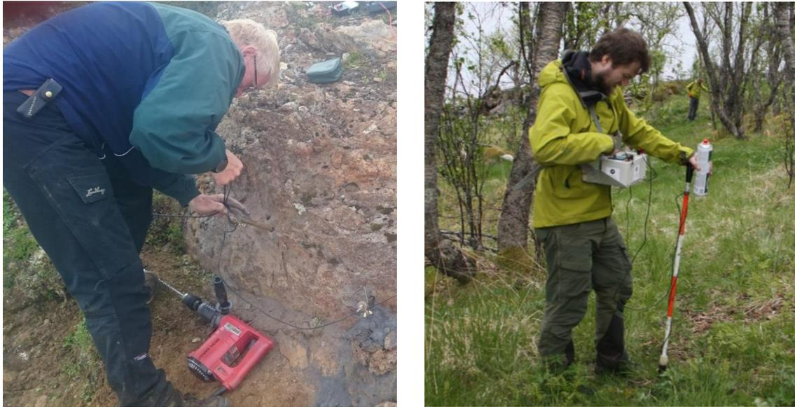
**Figure 4.4: Establishing CP ore-grounding point (left) and data acquisition in combined CP and SP data (right).**
