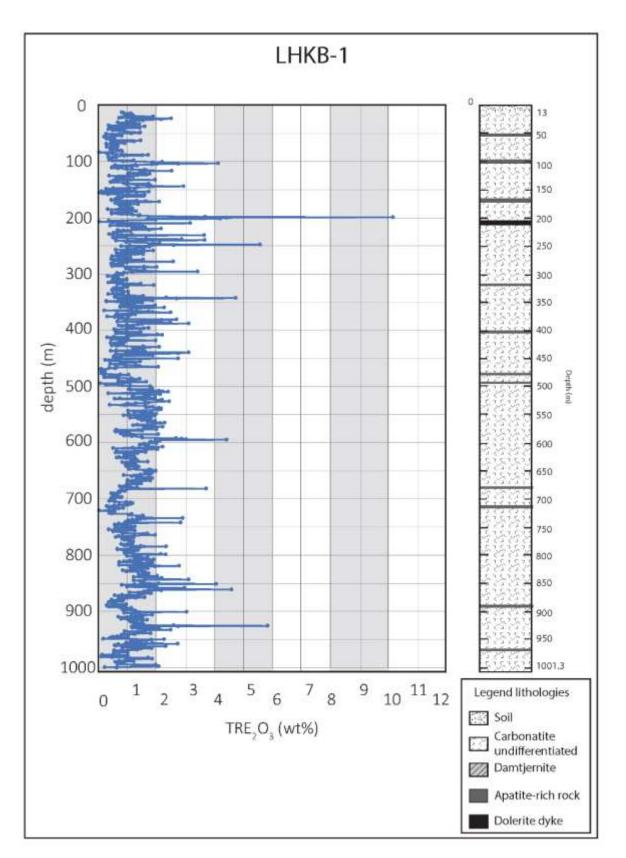
Figure 11: Total of Rare Earth Oxide in weight percent in LHKB-1.
