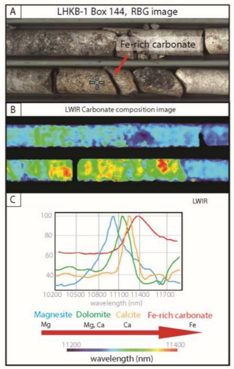
Figure 8: Carbonate compositional variations illustrated by LWIR data. A. Fe-rich carbonate (probably ankerite) in LHKB-1 core. B. LWIR carbonate composition image of the same area. C. Spectra of different carbonates encountered in carbonatite.
