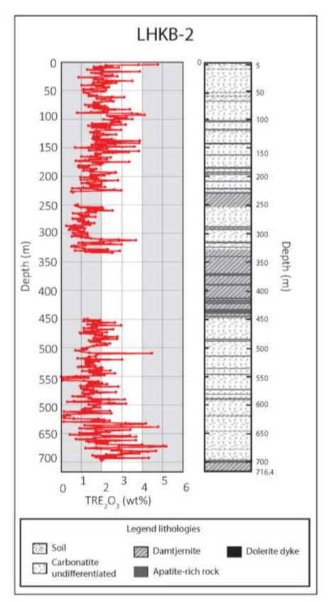
Figure 15: Total Rare Earth Oxide in weight percent in LHKB-2.
