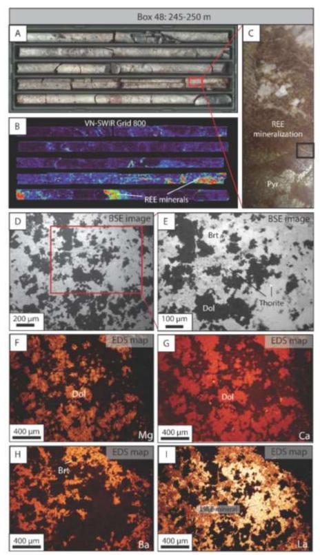
Figure 19: Texture of REE-mineralizations. A. Photo of the core box and location of the sample presented in this figure. B. Near Visible SWIR Grid 800 enhancing the location of REE-minerals in the core. D & E. Back Scattered Electron images of area mapped using EDS below. F to I: Energy Dispersive X-ray Spectroscopy maps showing chemical variation in the area presented in D.
