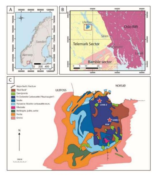
Figure 4: Simplified geologic map of the Fen Complex. A. Location of the Fen Complex in Norway. B. Simplified geologic map of the area (NGU 1:250 000 harmonized bedrock database). C. Simplified geological map of the Fen Complex.
