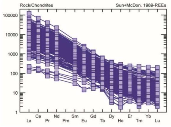
*Figure 13: Chondrite normalize REE diagram of samples from LHKB-1. Note the strong enrichment in LREE.*
