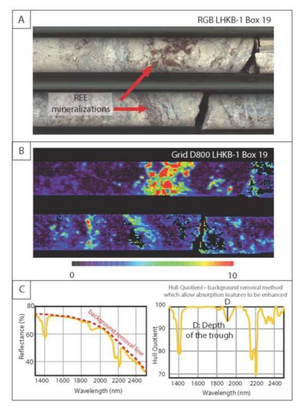
Figure 10: Grid D800 enhancing REE-minerals-related features. A. RGB photo of the core showing a zone enriched in REE-bearing minerals. B. Grid D800 image of the same part of the core as in A. C. Reflectance spectra and hull quotient background removal method (see text for explanation).
