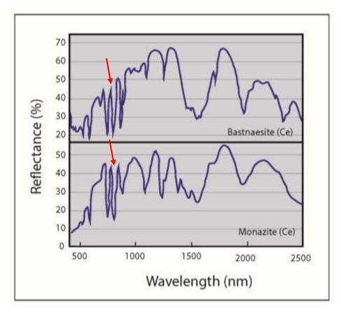
Figure 9: Reflectance spectra of REE-minerals encountered in carbonatite.
