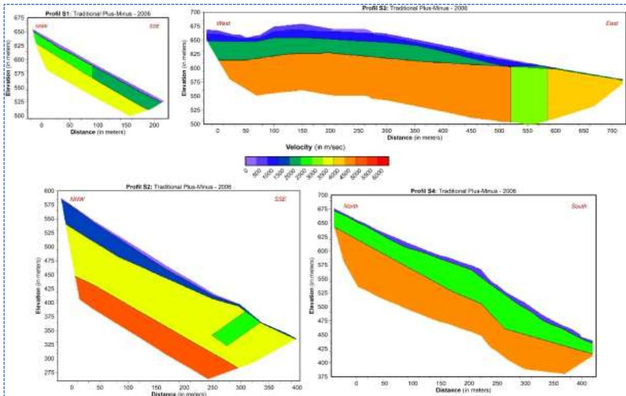
**Figure 6.1:** Digitized refraction seismic profiles S1, S2, S3 and S4 processed using traditional Plus-Minus method (Rønning, et al., 2006; Rønning et al., 2007).
