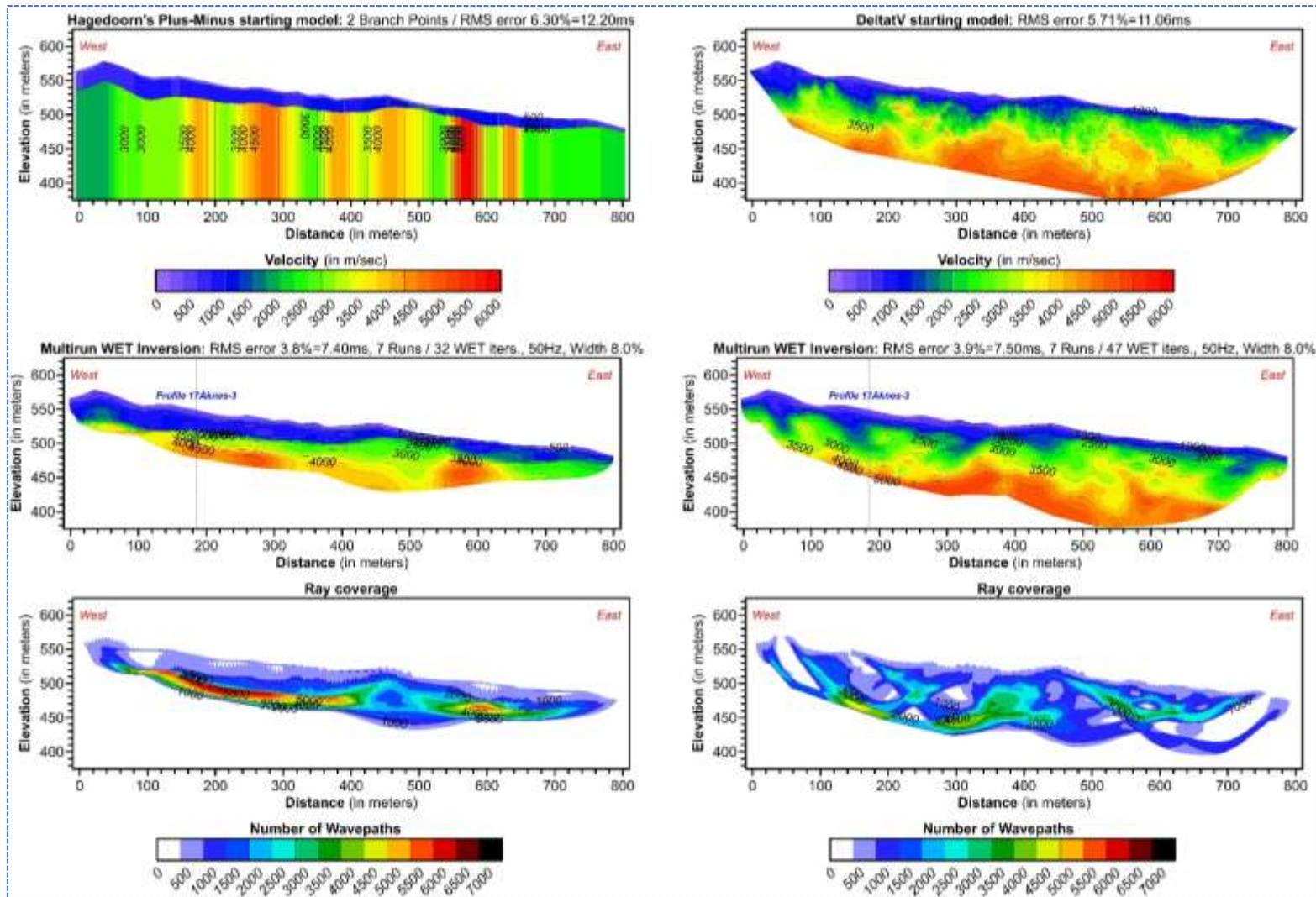
**Figure 4.1:** Profile 17Åknes-1 - Top: Initial models obtained by Midpoint Breaks and subsequent Hagedoorn's Plus-Minus application (left) and DeltatV (right) method. Middle: Multirun WET Inversion results using Hagedoorn's +/- (left) and DeltatV (right) starting models respectively. Bottom: Ray coverage for respective WET Inversion.
