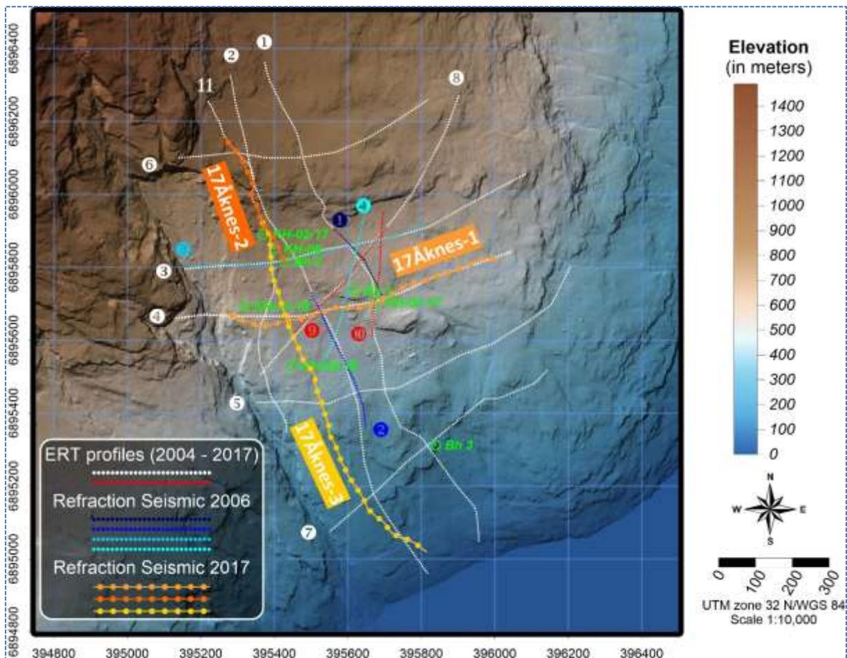
**Figure 2.1:** Positioning for all refraction seismic profiles conducted in Åknes in 2017 along with matching ERT profiles (white: 10 m electrode spacing, red: 5 m electrode spacing), refraction seismic profiles from 2006 and borehole positions. LiDAR elevation relief.
