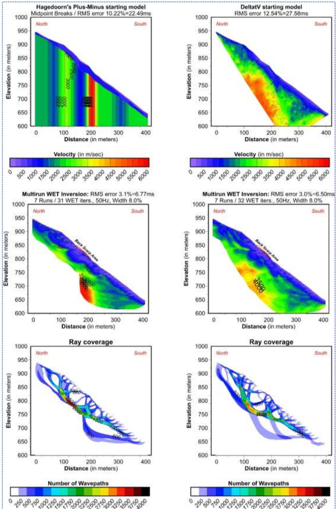
**Figure 4.2:** Profile 17Aknes-2 - Top: Starting models obtained by Midpoint Breaks and subsequent Hagedoorn's Plus-Minus application (left) and DeltatV (right) method. Middle: Multirun WET Inversion results using Hagedoorn's +/- (left) and DeltatV (right) starting models respectively. Bottom: Ray coverage for respective WET Inversion.
