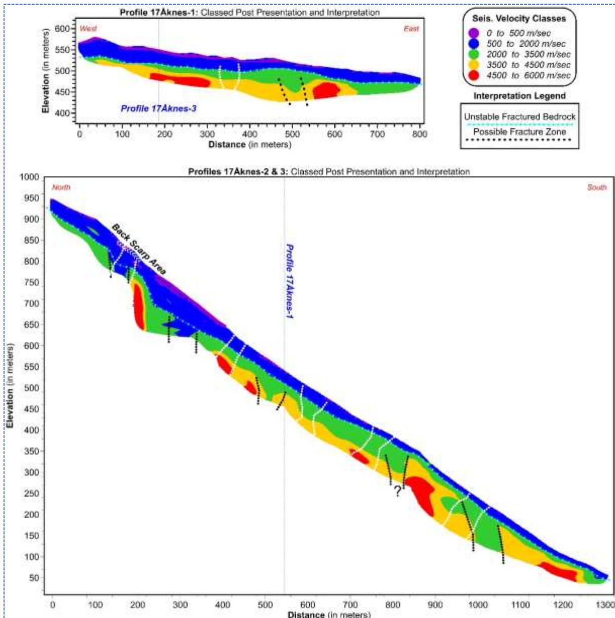
**Figure 5.1:** Classed post plotting of WET inversion acquired seismic velocities for all new seismic profiles in Åknes. Light blue lines: Interpreted top of fractured / water-saturated bedrock. Black dotted lines: Interpreted possible fracture zones from seismic data. White dotted lines: Possible fracture zones from resistivity data.
