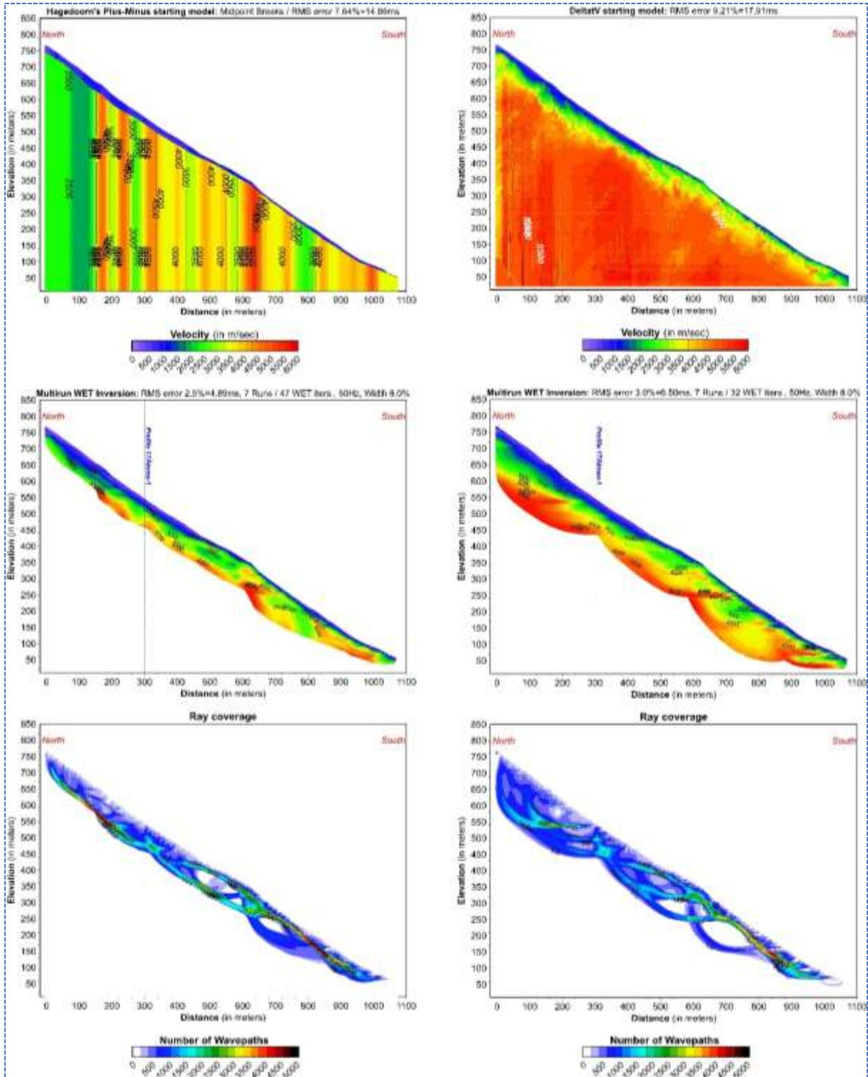
**Figure 4.3:** Profile 17Åknes-3 - Top: Initial models obtained by Midpoint Breaks and subsequent Hagedoorn's Plus-Minus application (left) and DeltatV (right) method. Middle: Multirun WET Inversion results using Hagedoorn's +/- (left) and DeltatV (right) starting models respectively. Bottom: Ray coverage for respective WET Inversion.
