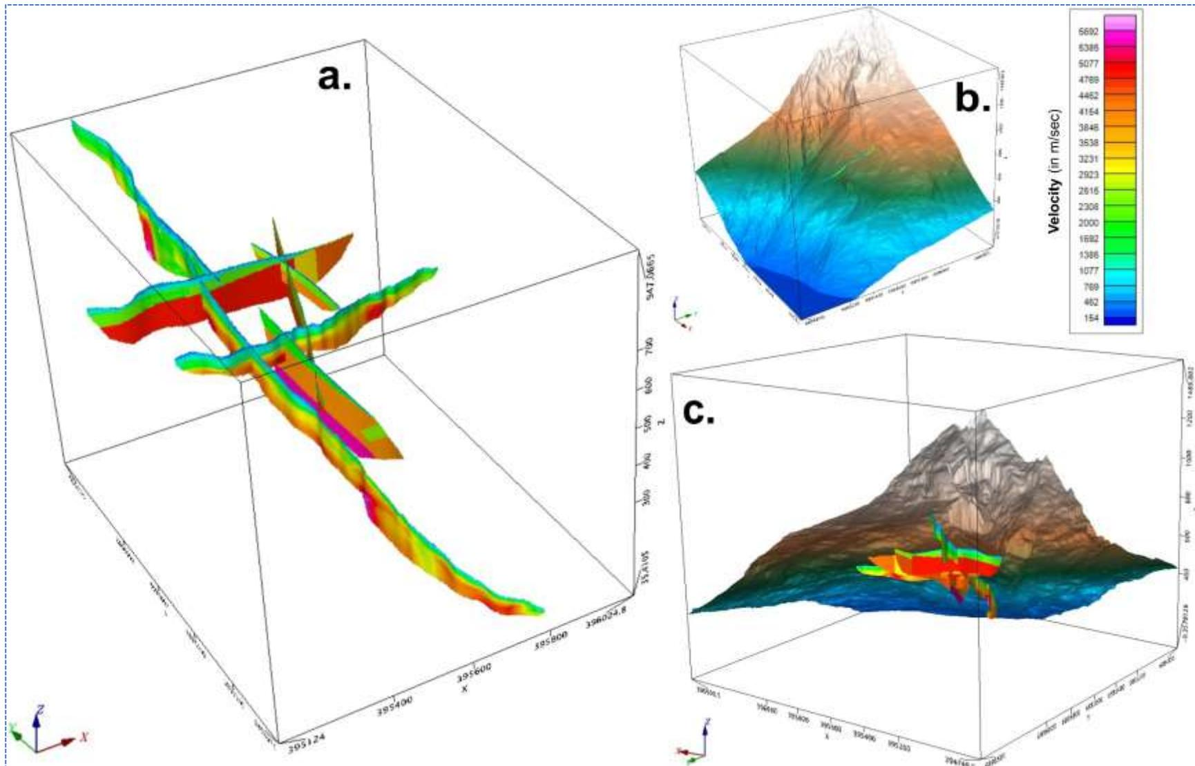
**Figure 6.2:** 3D presentation of the WET inversion and traditional Plus-Minus processed results from Åknes in Geosoft Oasis Montaj version 9.5. Coordinates in UTM zone 32 North and x, y, z axes in meters. (Azimuth View: a.  $33^\circ$  - SSW, b.  $305^\circ$  - SE, c.  $145^\circ$  - NNE).
