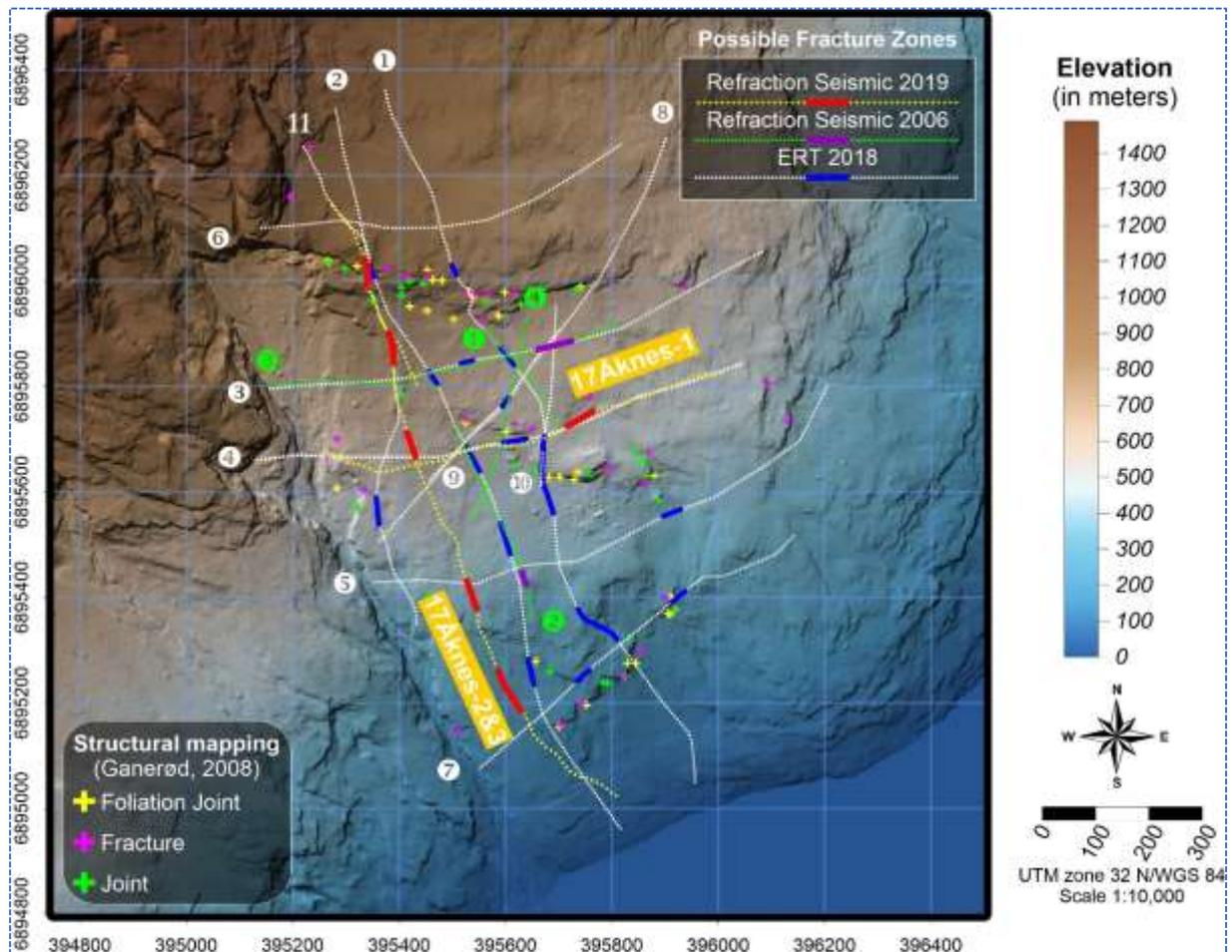
**Figure 5.2:** Positioning for all refraction seismic and ERT profiles conducted in Åknes along with interpreted fracture zones shown in colored boxes (red/violet and blue respectively). LiDAR elevation relief.
