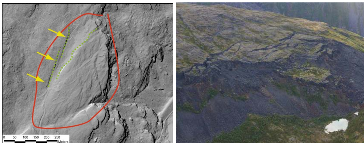
Figure 9: Left: Back scarp (yellow arrows) that is part of an opening graben (green dashed line) in back of large unstable rock slope indicated in red circle is only partly open in two segments. Right: Well developed scarps that do not connect to a singular back scarp (photo: H. Bunkholt). (The back scarp score would thus be 0.5.)
