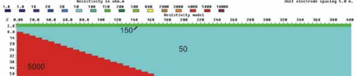
Figure 3.4.19: 3 m top layer (150 Ωm) over 50 Ωm and a dipping layer of 5000 Ωm. Standard inversion, V/H=0.5
