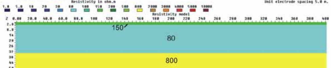
Figure 3.1.59: 3 m top layer (150 \Omega m) over horizontal layers of 80 \Omega m and 800 \Omega m. Standard inversion, V/H=0.5
