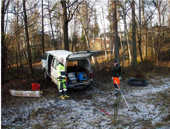
Figur 49. Logging i diamantborehull K 2.
