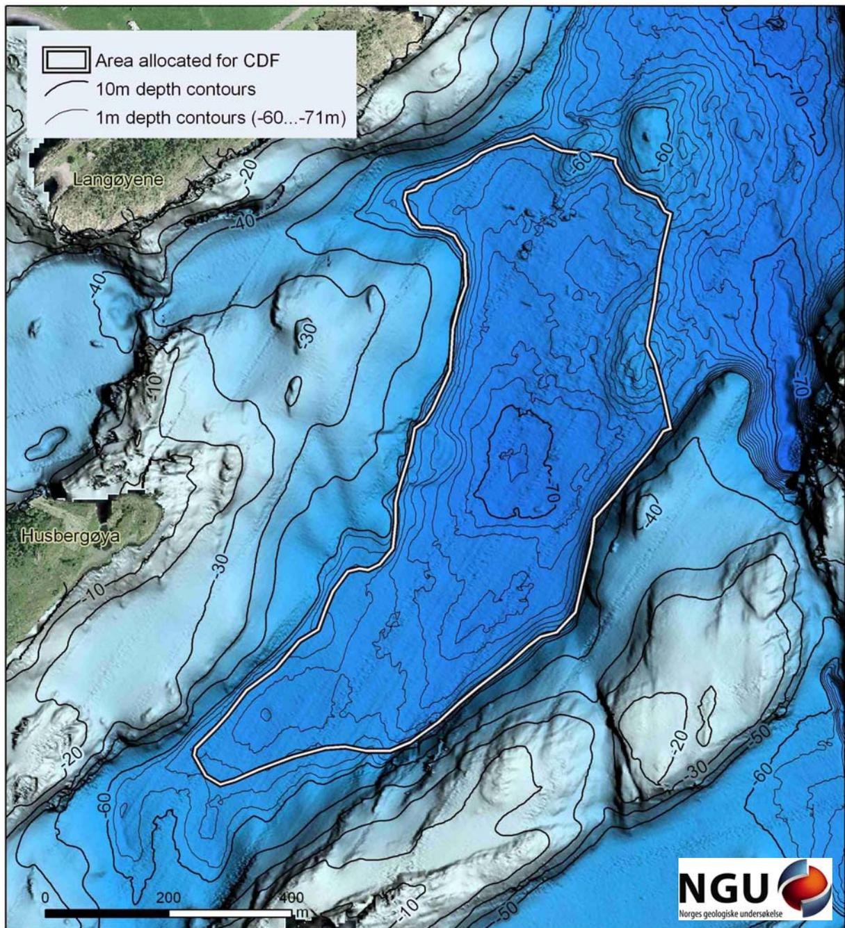
Figure 3. Depth-colored shaded-relief image with depth contours of the CDF area in 2004.
