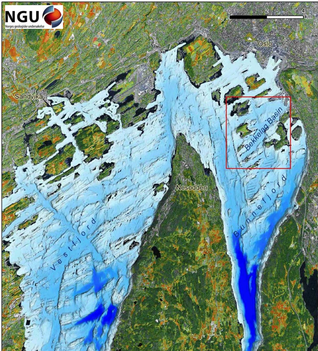
Figure 1. Depth-colored shaded-relief image of the northern part of the inner Oslofjord. Data are derived from the high-resolution bathymetric datasets collected by the Geological Survey of Norway (water depth 0-80 m) and the Norwegian Defense Research Establishment (water depth > 80 m). The red box gives the position of the Bekkelag Basin shown on Fig. 2 that is the study area treated in this report.
