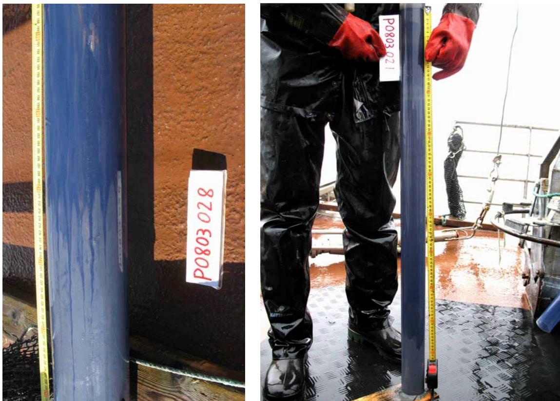
*Figure 7. Contact between dark gray disposed sediments and underlying olive gray original seabed sediments seen through the plastic liner in gravity (left) and Niemistö (right) cores.*
