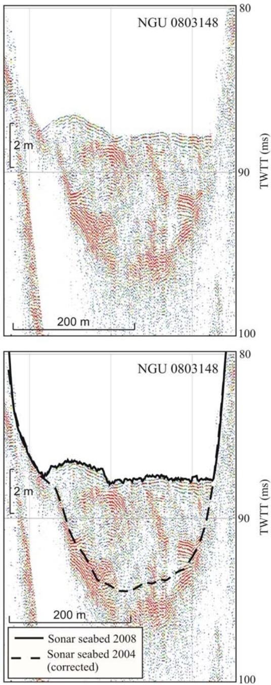
Figure 14. TOPAS seismic reflection profile (NGU0803148) across the CDF. Lower panel includes seafloor elevation lines from the 2004 and 2008 sonar datasets. Location of the profile is given on Fig. 6.
