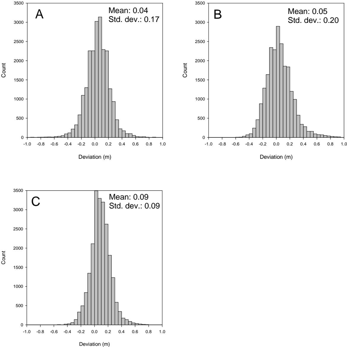
Figure 13. Histograms of seabed elevation differences between the 2004 and 2008 datasets in three reference areas of 22871 m<sup>2</sup> each (Fig. 9).
