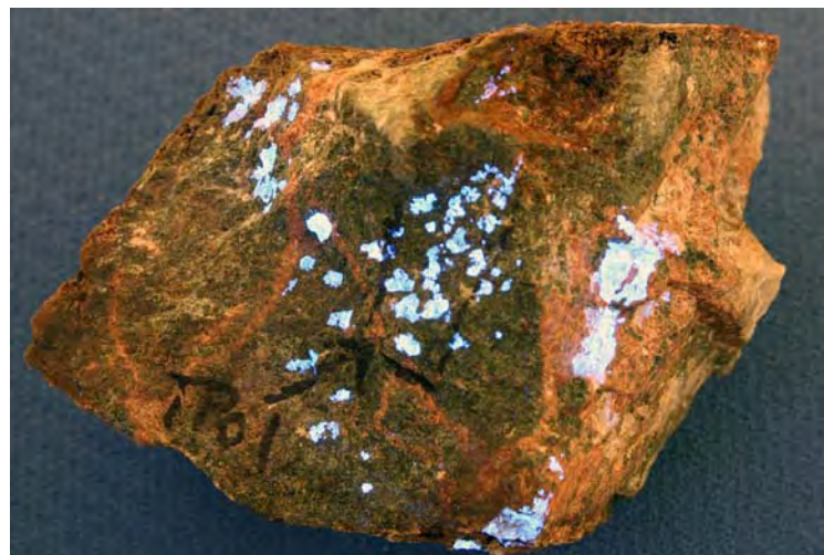
Figure 4. UV-light image of a garnet-diopside skarn with fluorescing scheelite crystals. The sample is 12 cm in length. Same sample (45462) as in Figure 3.
