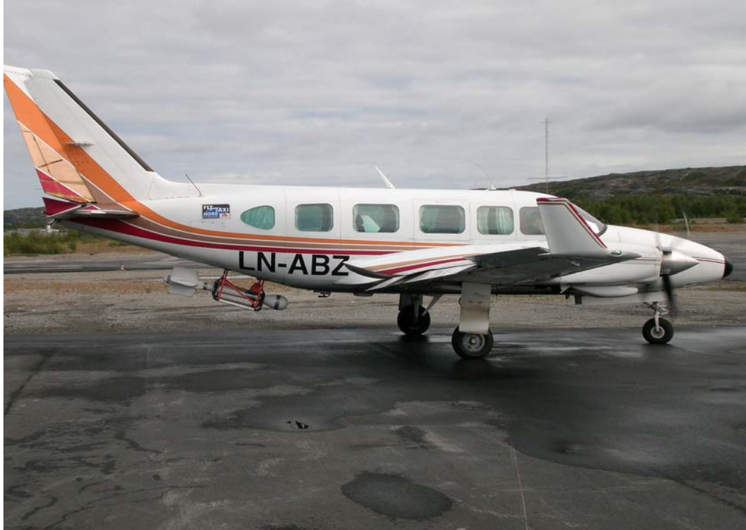
Piper Chieftain from Fly Taxi Nord with docking cradle for aeromagnetic sensor.
