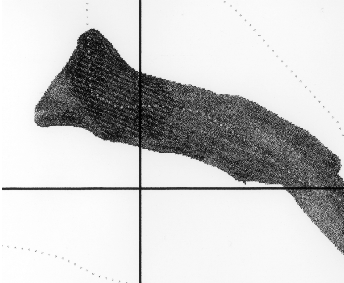
Figure 10. Screen dump of backscatter mosaic from Møre. The histogram function has been applied two times, with a correction factor of 90%. The mosaic has a reflectivity between -60 dB to -5 dB. The stripe effect is present throughout the survey area, but is most prominent within the till area in Haramsfjorden, as shown. The area is approximately 5 km from east to west.
