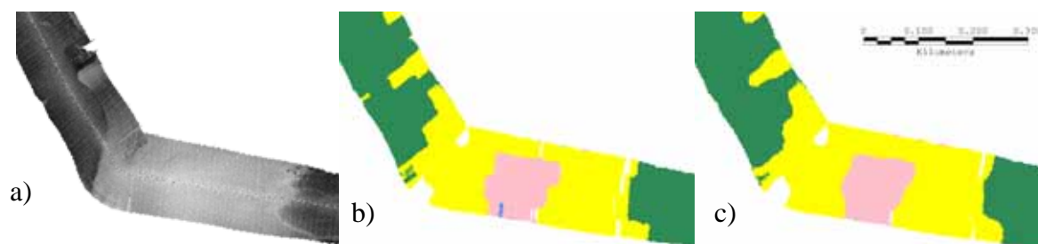
Figure 8. Backscatter mosaic and automatic interpretation of a single multibeam line acquired using an EM1002. a) Backscatter mosaic created using Poseidon. b) Automatic interpretation using Triton and subsequently using a filter size of 5. c) Same interpretation as in b, but using a filter size of 15.
