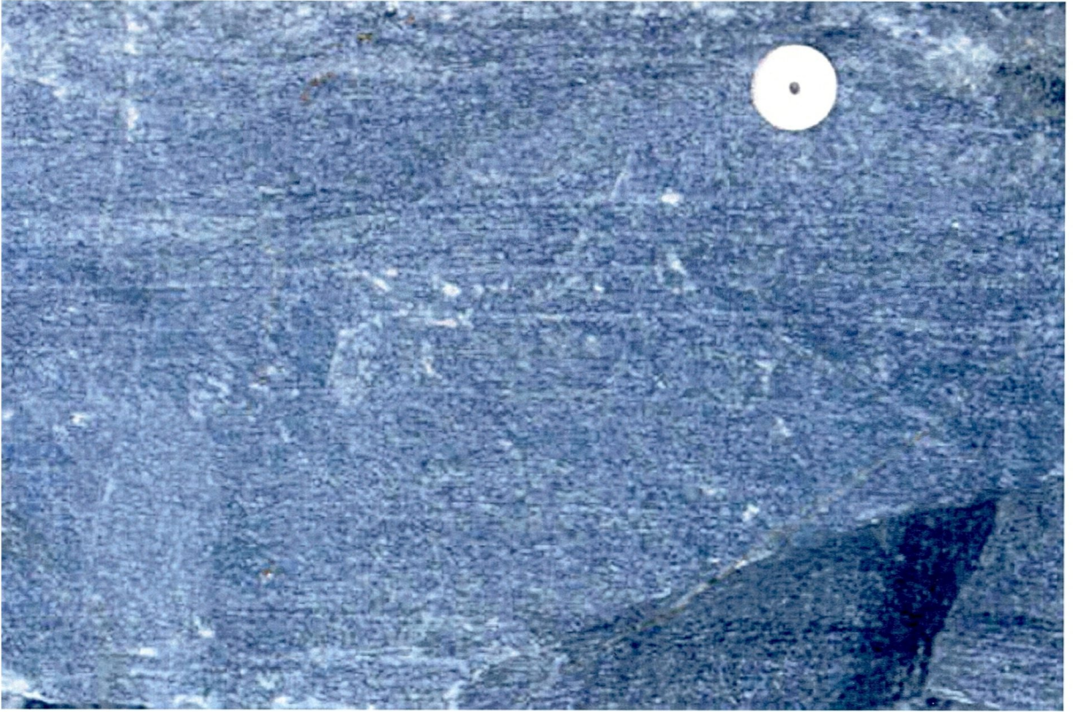
Fig. 2. Fine-grained grey gneiss; diffusely banded and foliated. Coin diameter 26 mm.
