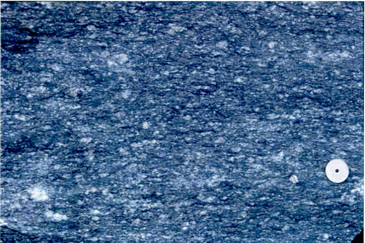
Fig. 4. Well-foliated, mylonitic porphyritic granodiorite with drawn-out feldspar phenocrysts. Coin diameter 26 mm.
