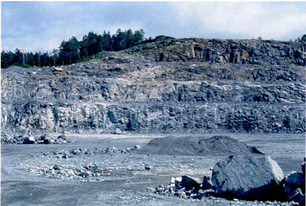
Fig. 7. Zone III in northern part of present quarry consisting of porphyritic granodiorite with lenses of fine-grained grey gneisses (both dark). 3-5 metres thick sheets of pegmatites (three different levels) show with pale colour in the left part of the picture. View to northeast from level +17 m.
