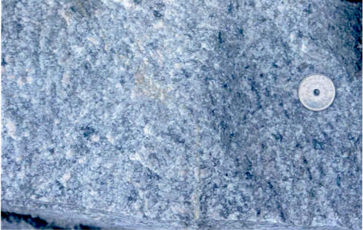
Fig. 5. Pale grey granite; weakly foliated although gneissic. Coin diameter 26 mm.
