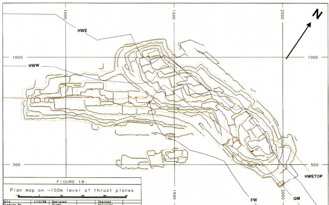
Figure 9: Plan map of the Björkdal Mine with the projected intersections of mapped thrust structures on the -100m bench level.
