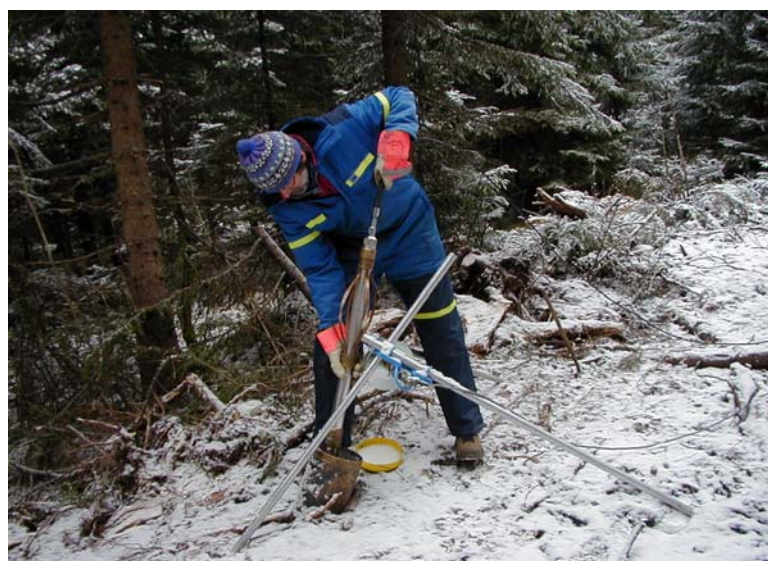
Figur 3. OPTV sonde klar for logging i Bh 6.
