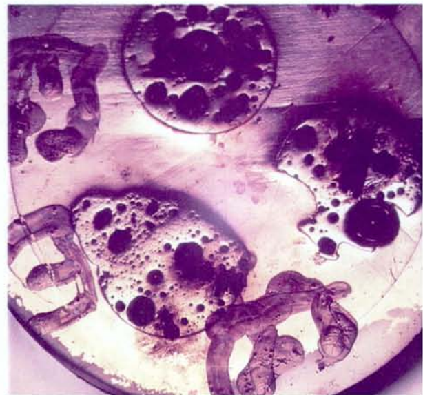
Figure 3: A) Ablation crater by in situ ablation of quartz with a beam diameter of 30\ \mu\text{m} that also corresponds to the approximate diameter of the crater; here shown in reflected light at high magnification. Notice how it is possible to identify individual sub- \mu\text{m} droplets of silicate melt along the crater rim. They were produced during the ablation. B) Ablation crater that in contrary to (A) was produced during ablation over an area in which the UV-laser operates according to a predefined grid. The crater shown on (B) was produced at Monash University and with approximate dimensions of 800 \times 350\ \mu\text{m} , they are much larger than the 250 \times 250 grids produced at NGU. The dark shadow surrounding the crater comprises silicate melts that were produced during the ablation process. C) Custom made quartz standards produced at NGU by M. Ødegård et al. (1998). The standards are ca. 5 mm in diameter. Dark areas are vesicles.
