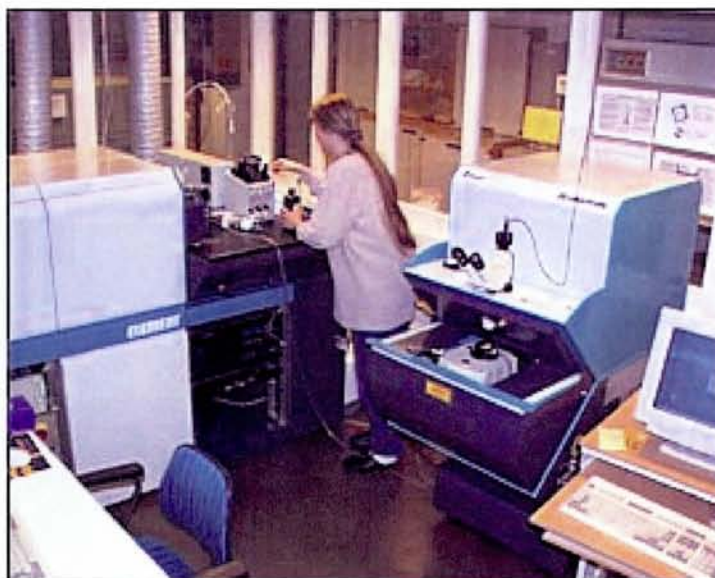
Figure 4: The picture above show the LA-HR-ICP-MS instrument at the Geological Survey of Norway. To the left, is the Finnigan MAT ELEMENT double focusing, sector field mass spectrometer. To the right is the Finnigan MAT-Spectrum UV-laser. The protection shield around the laser unit is open so that one may have a look into the sample chamber (black well on the white block), where the quartz samples are inserted before analysis. A tubing system (not visible) running behind the operator conveys the ablated material from the laser unit to the mass spectrometer.
