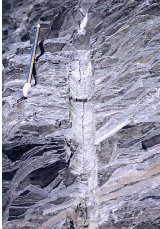
Fig. 5.3.6. Axial fracture in a borehole wall at Skogvika, Laksefjord, in Friarfjord Formation phyllites with silstone layers; looking northwest. Indications of borehole offset can be seen to the right of the pencil (hanging-wall coming 'up', out of the picture).
