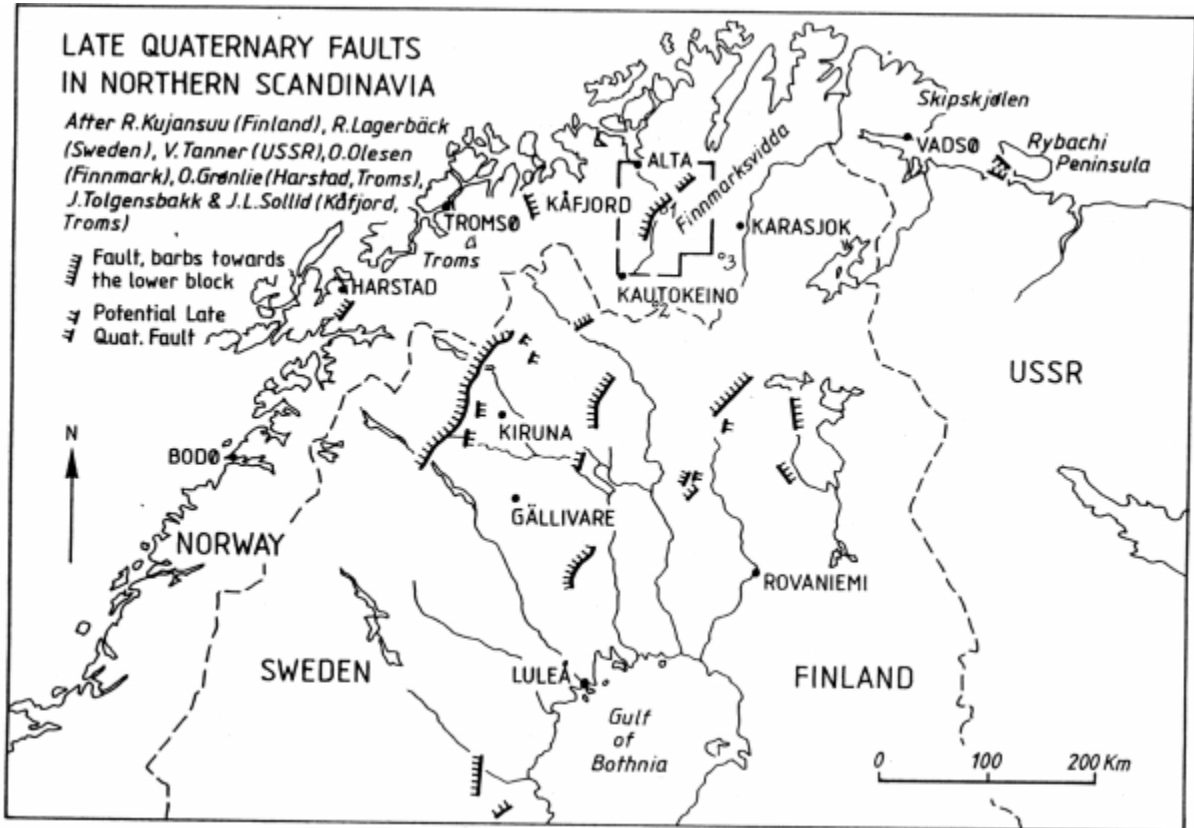
Fig. 5.2.1. Late Quaternary faults in northern Fennoscandia. The area covering the Stuoragurra Fault (Fig. 5.2.2) is framed. 1 – Masi, recent earthquake. 2, 3 – Till avalanches, possibly earthquake initiated. Mainly after Olesen et al. (1992a).
