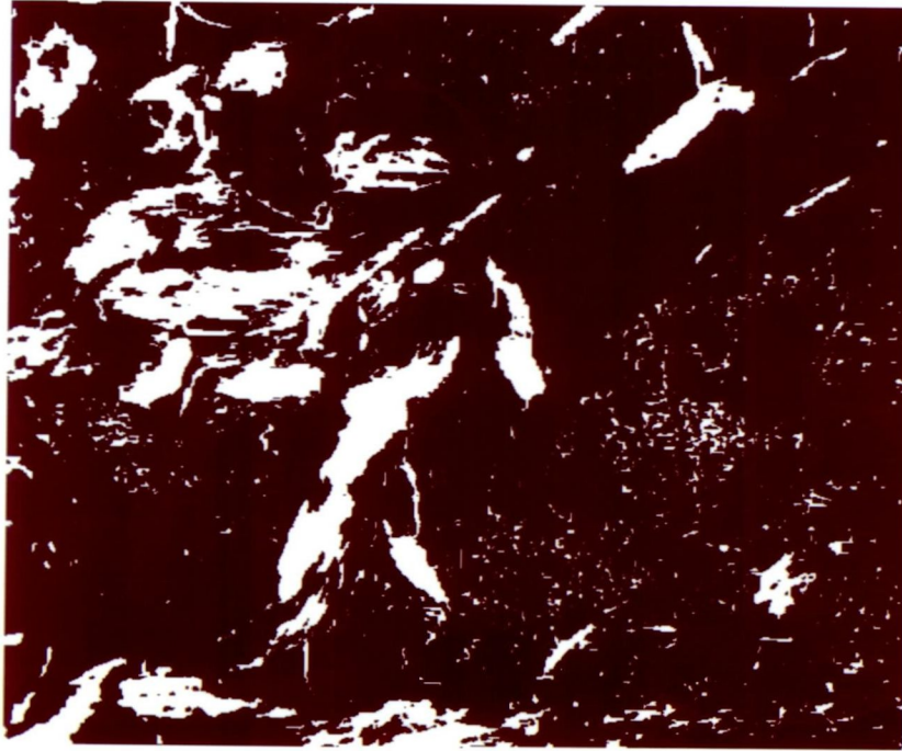
Figure 7 Binary image, with opaque phases of fig 6 is shown in white
