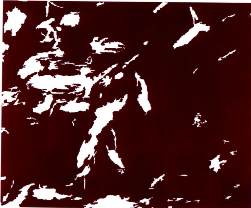
Figure 8 Processed binary image where small objects are eliminated
