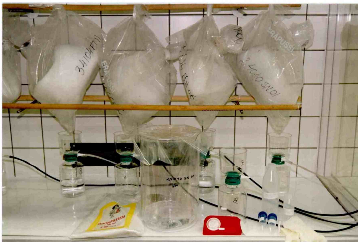
Fig. 5: Overview of the system used for on-line melting and filtering of snow.
