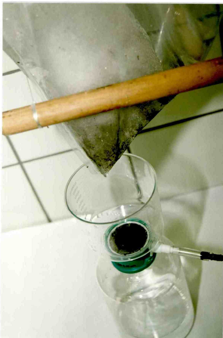
Fig. 6: Concentration of soot and particulates at the bottom of the PE-bag during the melting process.
