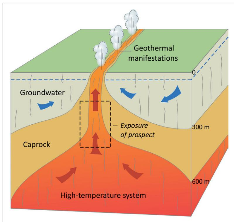
Figure 5. Conceptual model of the Mogilsa geothermal system (modified from Franzson et al. 1992).
