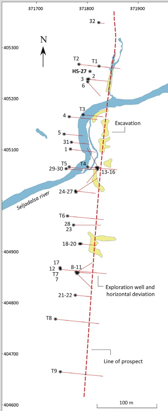
Figure 6. Map showing the alignment of the quartz-adularia vein and the location and horizontal projection of the 41 drillholes at Thormodsdalur. Excavation north of the river shown in Figure 8 (modified from Fleming et al. 2006).
