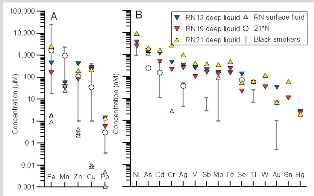
Figure 11. Metal and trace-element concentrations (in  $\mu$ Moles and nMoles) from three wells in the Reykjanes geothermal system compared to black smokers (21°N EPR, TAG and 5°S at MAR) (Hardardottir et al. 2009).
