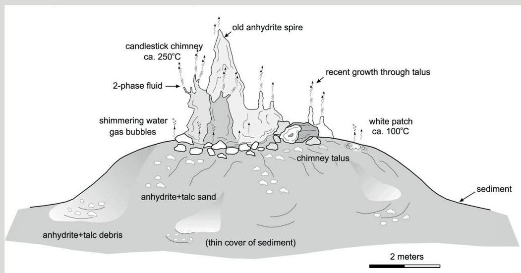
Figure 15. Sketch showing the main characteristics of an anhydrite hydrothermal mound found at Grimsey hydrothermal field (Hannington et al. 2001).
