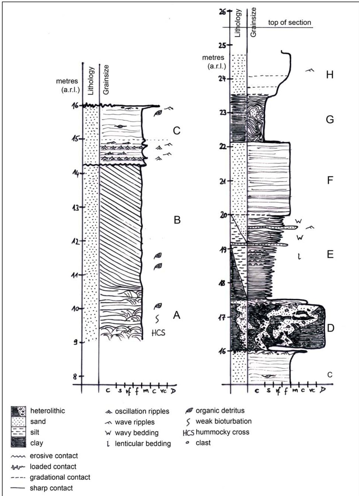
Fig. 14. Sediment log of the profile at Tolokonka Loc.06025, 3.24 km downstream Severnaya Dvina. Letters A to H indicate the different units that have been described. Elevations are given in metres above river level (a.r.l.).
