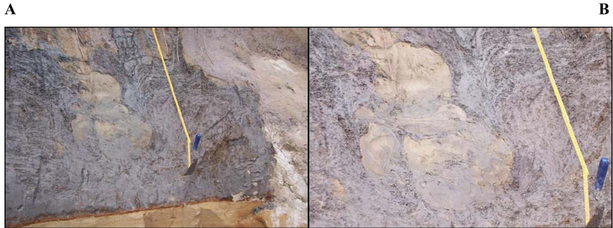
*Fig. 30. A) very wet, deformed laminated clay unit G. B) preserved lamination in the clay. Sand is worked into the deformed unit G. Pictures are orientated NW-SE.*
