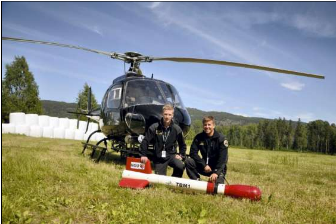
Figure 4: Photo of Heliscan's Eurocopter AS350-B2 (P1). The Mag bird in front of the helicopter and the spectrometer under its belly are also depicted.
