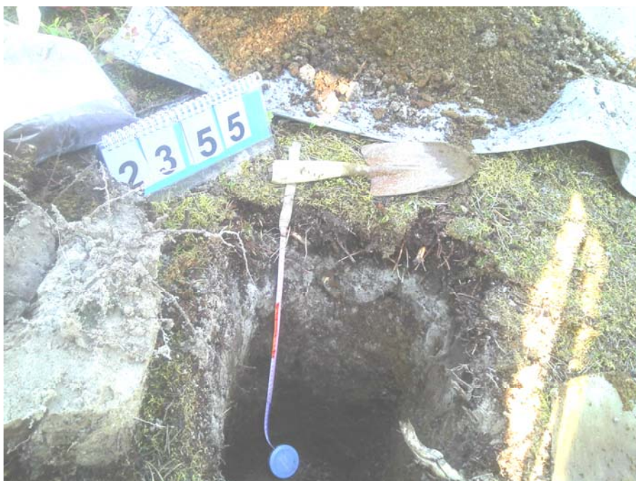
Figure 3. Typical sample pit with sampling tool and sample.
