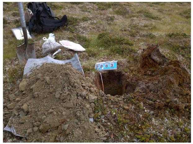
Figure 3: Photo showing sample, sample pit and all essential tools. Photo O.A. Eggen
