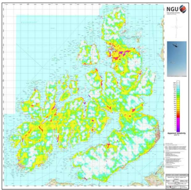
Figure 9: Apparent resistivity. Frequency 880 Hz, Coplanar coils
