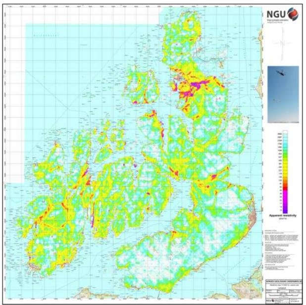
Figure 10: Apparent resistivity. Frequency 7000 Hz, Coaxial coils
