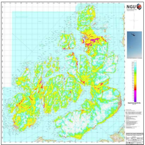
Figure 8: Apparent resistivity. Frequency 6600 Hz, Coplanar coils
