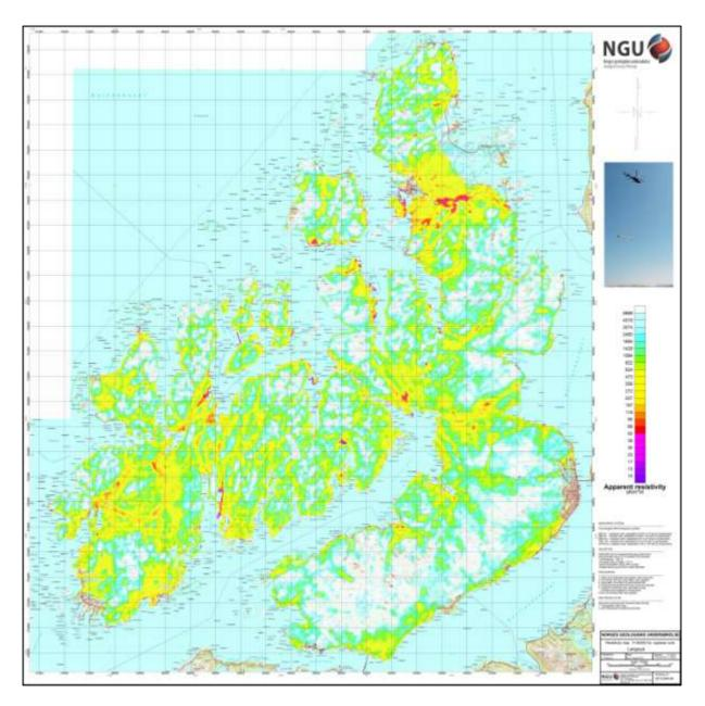
Figure 7: Apparent resistivity. Frequency 34000 Hz, Coplanar coils
