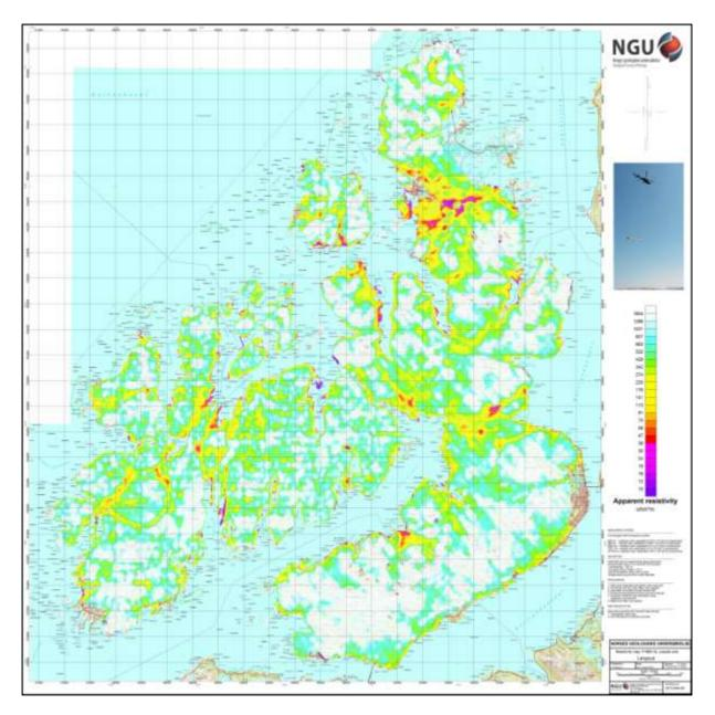
Figure 11: Apparent resistivity. Frequency 980 Hz, Coaxial coils
