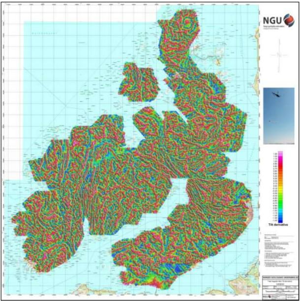
Figure 6: Magnetic Tilt Derivative
