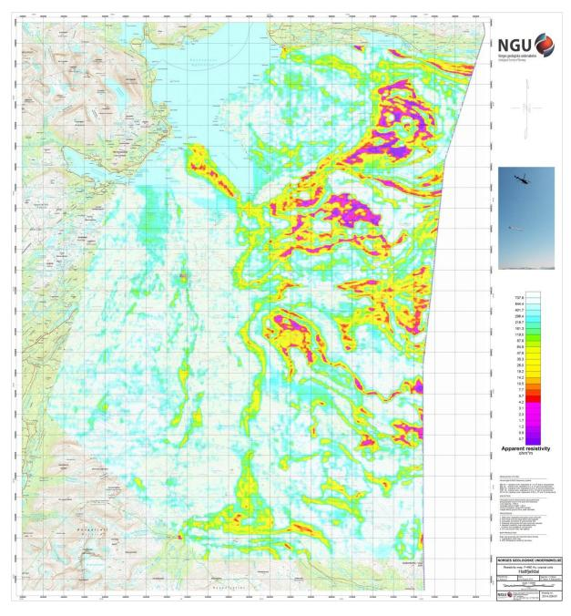
Figure 11: Apparent resistivity. Frequency 7000 Hz, Coaxial coils
