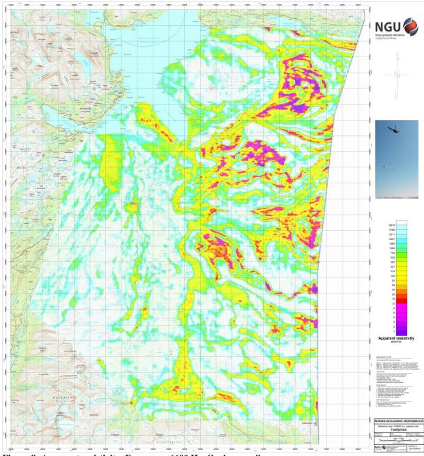
Figure 8: Apparent resistivity. Frequency 6600 Hz, Coplanar coils
