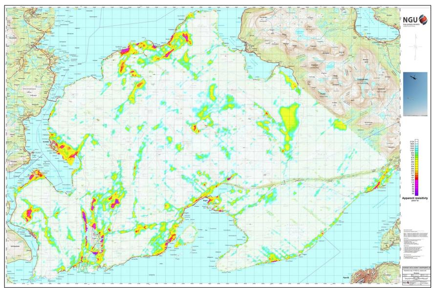
Figure 10: Apparent resistivity. Frequency 7000 Hz, Coaxial coils
