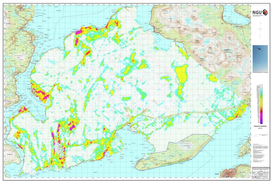
Figure 7: Apparent resistivity. Frequency 34000 Hz, Coplanar coils
