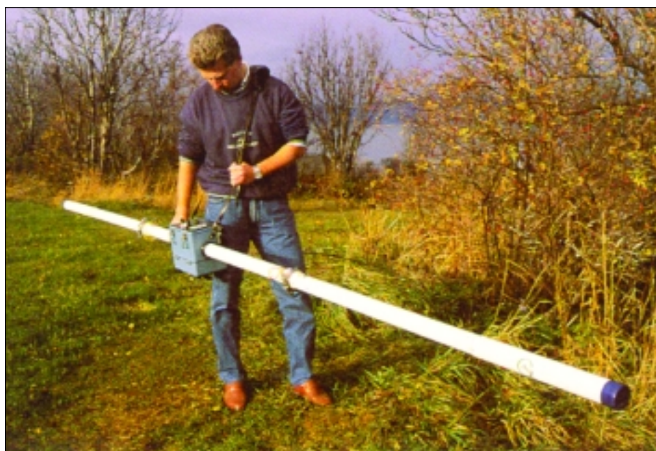
Figure 13. (a) The use of electromagnetic induction (EM31) equipment in the field to measure conductivity (photo: Ingemar Aamo); (b) a Georadar profile and its interpretation, showing the bedrock surface below superficial deposits (hatched) and low angle fractures in the underlying bedrock (from Hvaler, Norway - Banks et al. 1993b)
