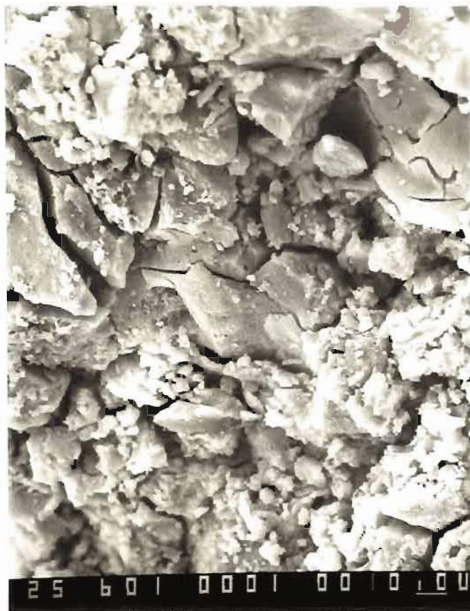
Rough and smooth surface: Fe-phases (with minor Mn)
