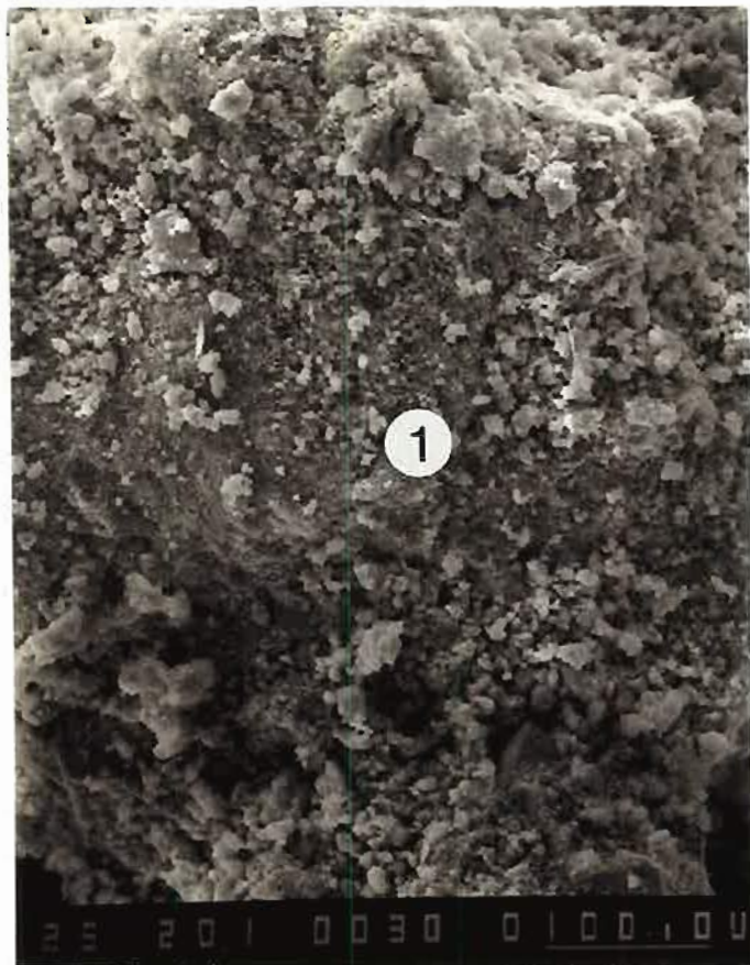
Rough surface: Fe-phase (with minor Mn)
