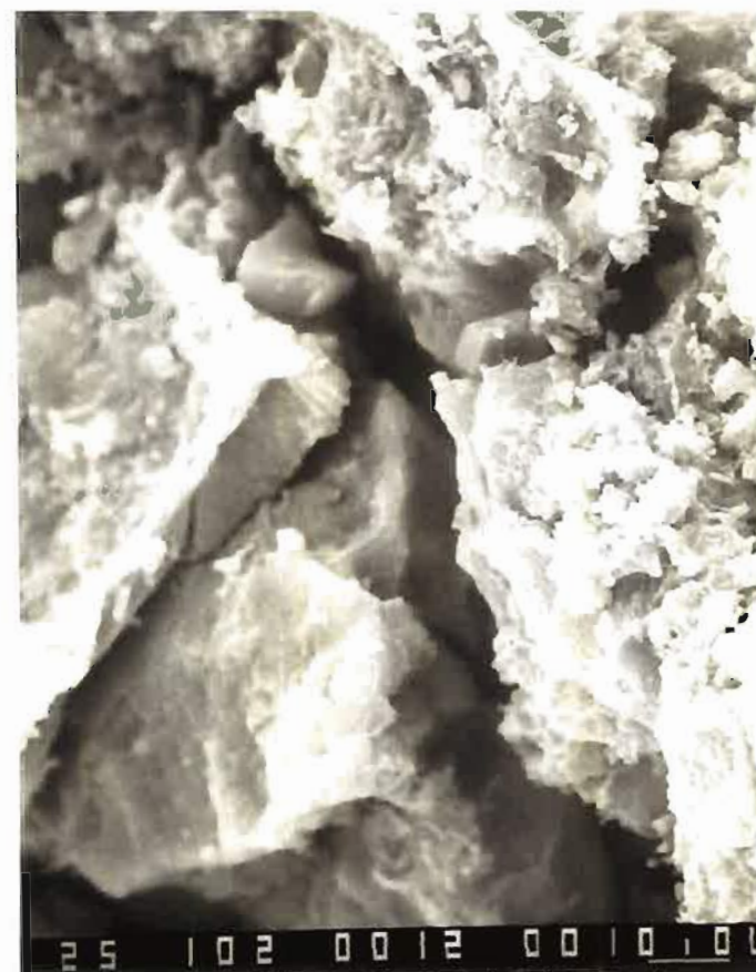
Rough surface: Mn-phase
