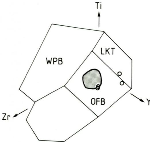
Fig. 22. Simplified Ti-Zr-Yi diagram showing the plots of 4 analysed gabbro samples (circles) from the lower tectonic unit. The field with grey ornament embraces samples of mafic dykes from the upper tectonic unit (Zwaan & Roberts 1981, Roberts 1990). The gabbro analyses were carried out in 1987 at NGU using a Philips PW1404 XRF spectrometer. The complete analytical data from the gabbro samples can be obtained from the first author upon request.
