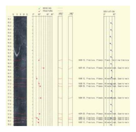
Optical televiewer drill hole log. Left image of drill hole (80 mm in diametre) projected to a flat surface. Interpretation of joint surfaces (directions, groupings and spacing) and layering is done semiautomatically. Source: Geological Survey of Norway (NGU).
