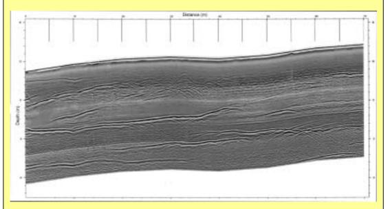
GPR section from a Finnish granite quarry, showing clearly the horizontal fractures.
