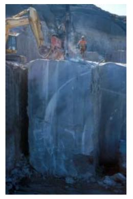
Slicing a loose primary block. "Labrador Antique" quarry, SW Norway.
