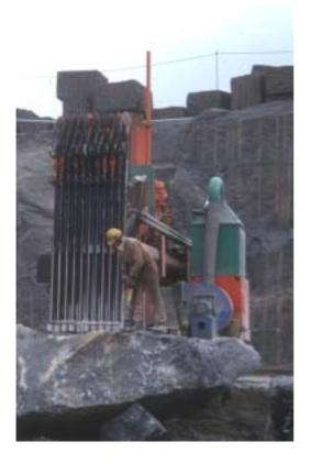
Multi-hammer, hydraulic driller for squaring of blocks.
