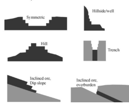
Schematic drawing showing some different open-cast situations. Workable part of deposit shown in black.
