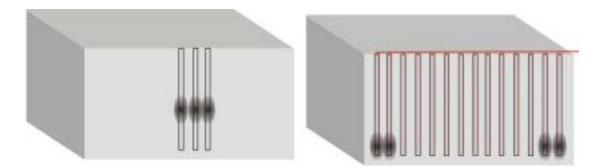
Two examples of granite splitting with the use of black powder. Left: black powder (dark spots) in three central holes placed along the primary cleavage plane of the granite. Right: black powder only in the marginal holes, combined with detonating fuse (red line)
