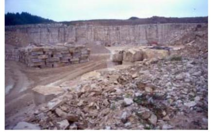
Only the lowermost part of this limestone formation in Germany is usable for ornamental stone. The rest is applied for aggregate and cement.
