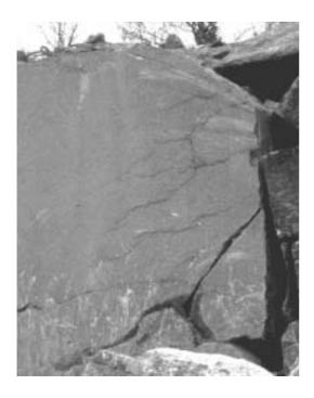
Figure: damages (cracks) from blasting
