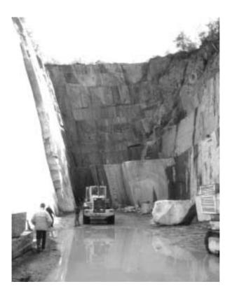
Trench-quarry, "Serizzo"gneiss, Northern Italy. Note that the layering (foliation) of the rock is almost vertical.
