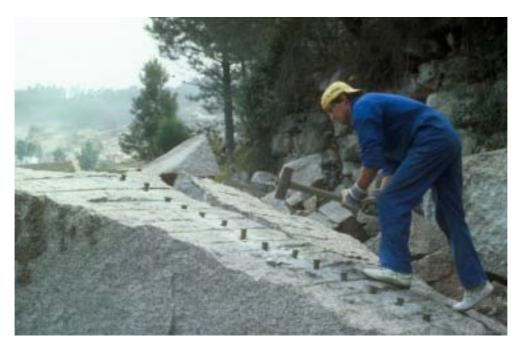
Worker using short plugs for wedging granite block in Vigo, Spain.
