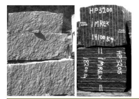
Rough granite blocks squared with short wedges (left) and long "plugs and feathers". The former granite is far more brittle and easier to split than the latter.
