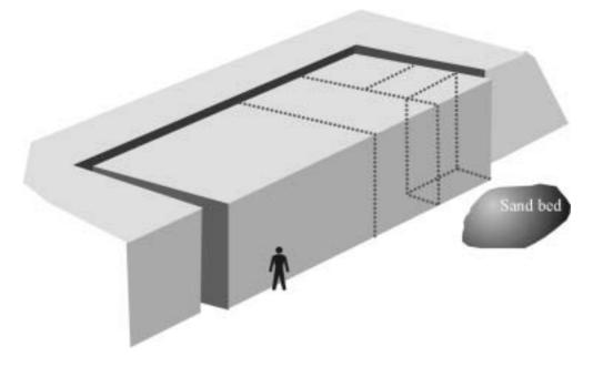
*Principle of block extraction – from primary blocks to smaller sized slices, which will be further divided to commercial blocks.*
