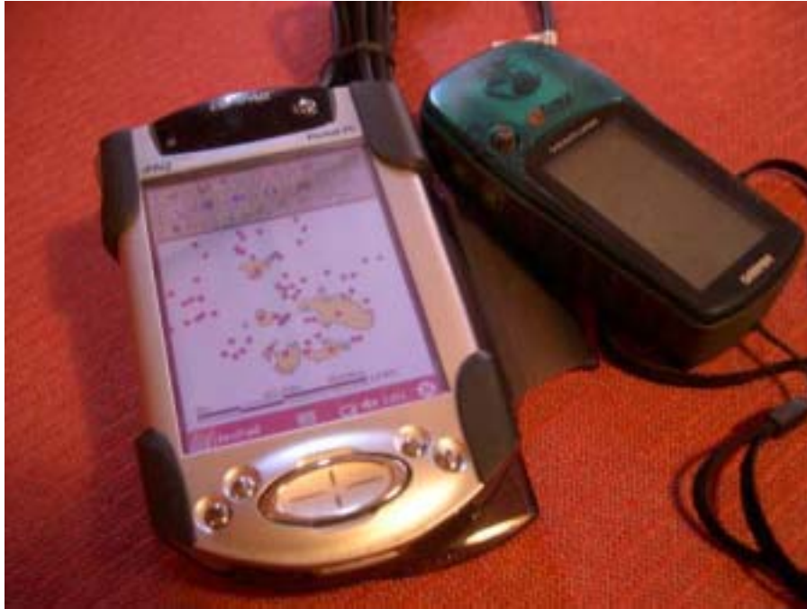
Figure 7: Ipaq pocket computer connected to a Garmin eTrex Venture GPS was used for mapping in the field.
