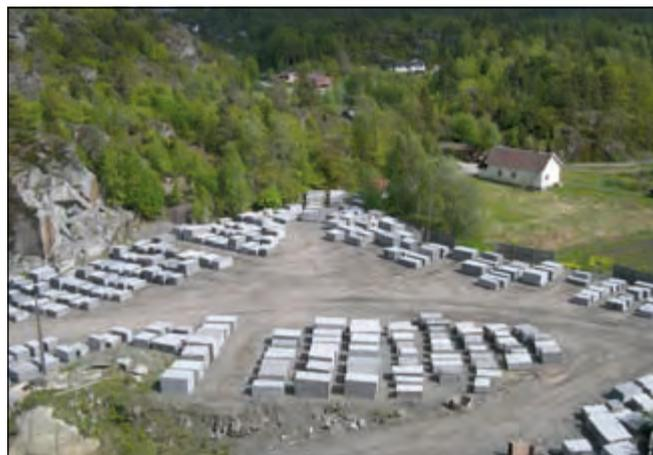
Figure 4. Stock of larvikite blocks at Tvedalen ready for shipping abroad.
