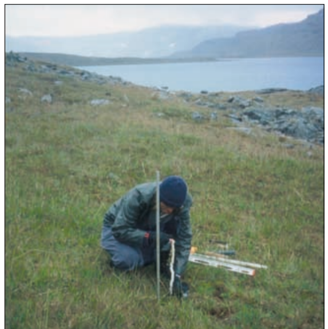
Figure 10. Installation of depth-integrating peg profile at a solifluction lobe in Latnjavagge.
