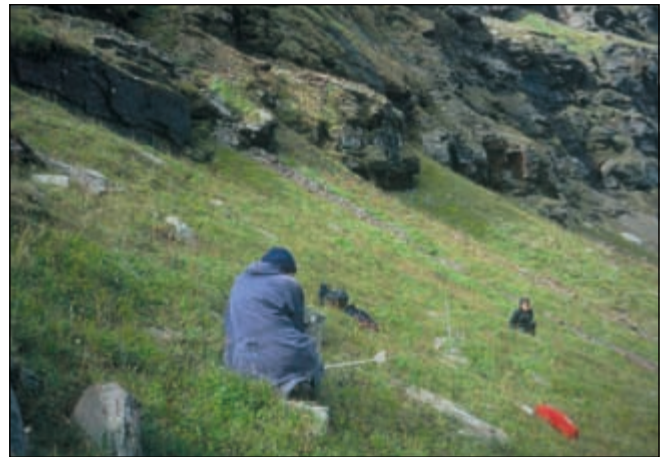
Figure 9. Monitoring of creep processes with painted stone lines and steel-rod lines at a slope test site in Latnjavagge.
