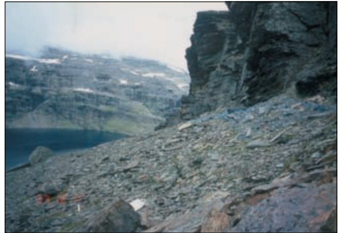
Figure 8. Monitoring of creep processes with painted stone-tracer lines and steel-rod lines at a talus cone/slope test site in Latnjavagge.
