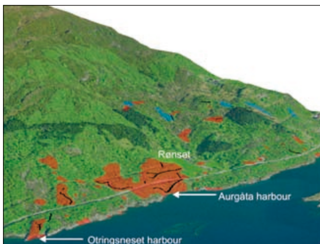
Figure 4. Perspective model of the Rønset quarry area, Hyllestad (Rønset farm is seen in the centre of the image). Red colour: quarries where millstones have been carved directly from bedrock, blue colour: quarries where blasting was applied for primary extraction. Black lines are ancient quarry roads and tracks.
