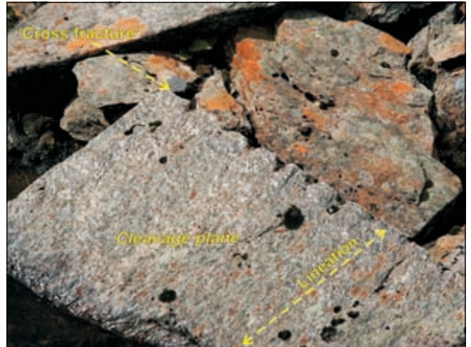
Figure 14. Close-up of slab from a quarry in the northwestern part of Hogfjellet, Selbu, showing a cleavage plane with lineation marked by a characteristically undulating surface. The slab was loosened along the primary cleavage using chisels and pick-axe (note tool marks) on a free 'cross-fracture' plane marked on the photo. The left side of the slab was broken along the lineation as discussed in the text.
