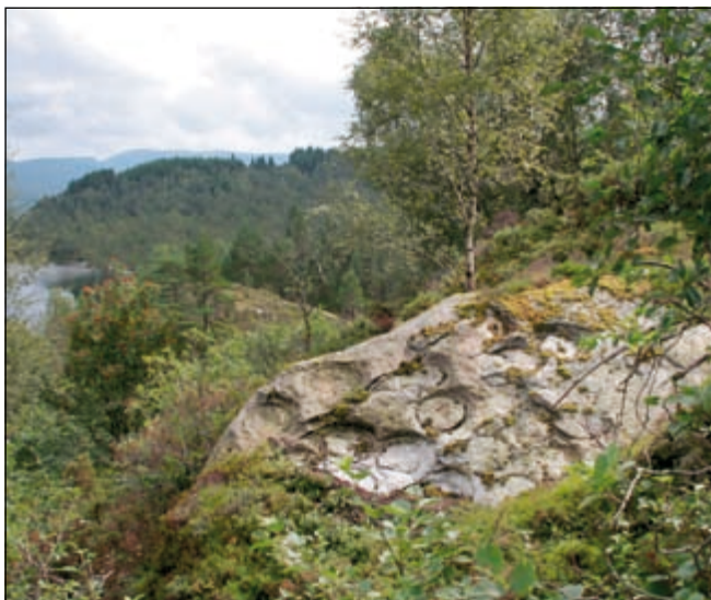
Figure 19. Shallow quarry established in layers along the cleavage plane, Sesol area, Hyllestad.
