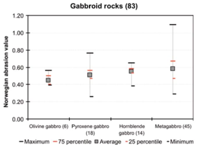
Figure 11. Effect of alteration on the Norwegian abrasion value for gabbroid rocks. Number of analyses in parentheses.
