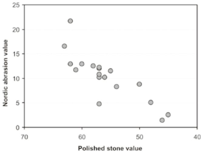
Figure 13. Polished stone values vs. Nordic abrasion value for sandstones.
