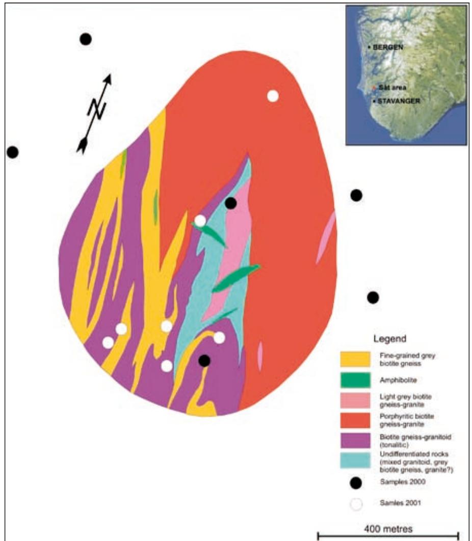
Figure 2. Geological map covering the potential extraction area of Sât (Marker and Erichsen 2002).
