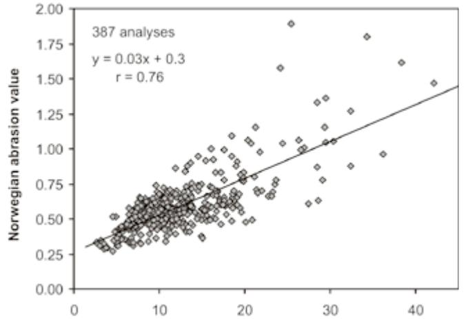
Figure 10. Nordic abrasion value vs. Norwegian abrasion value. Analyses from NGU's Database for hard-rock aggregates.
