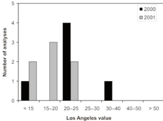
Figure 3. Variation in the Los Angeles value for samples collected in 2000 and 2001 from the potential extraction area of Sât (Marker and Erichsen 2002).
