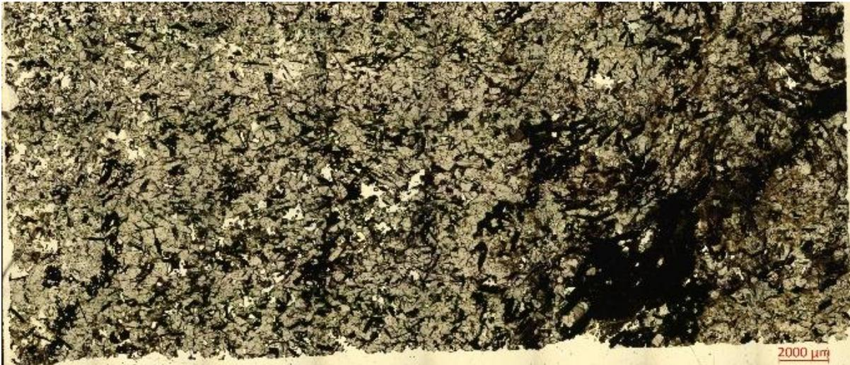
Figure 6.13: Thin section JK-DhSom1701-19.7, host rock that contain graphite in veins and disseminated thin long graphite flakes and abundant iron sulphides.
