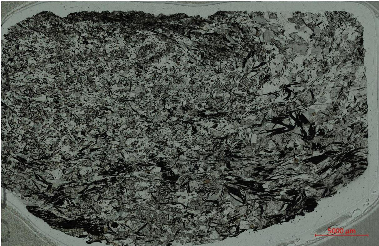
Figure 12.3: Thin section of graphite bearing rock showing large variations in both grain size and amount of graphite crystals over short distances (thin section JK6617-2).
