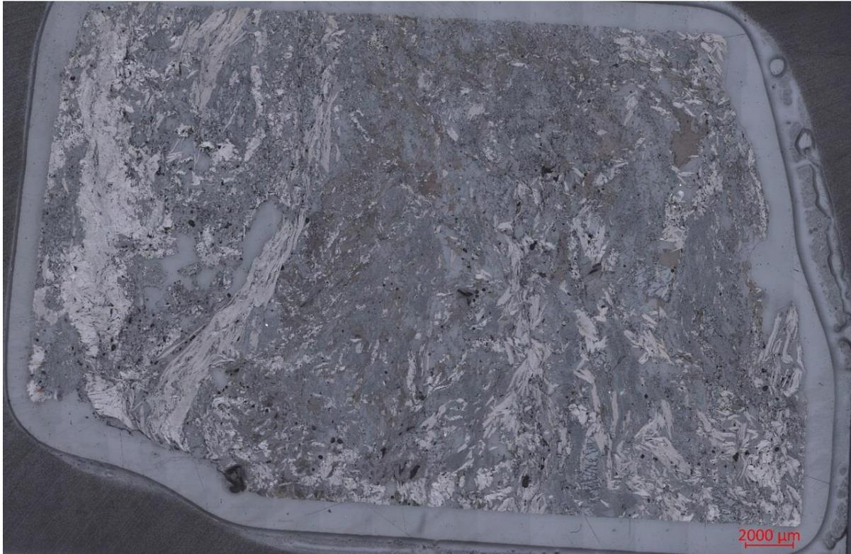
Figure 12.2: The graphite seen in reflected light showing large variations in the distribution and grain size of graphite flakes (thin section JK-2617-2-Sommarhus- 24,7%TC).
