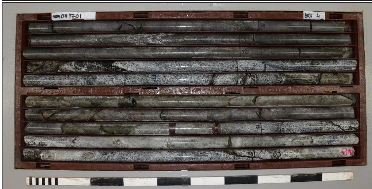
Figure 6.9: Part of drill core (dry upper and wet lower picture) showing a sequence with graphite schist, impure marble (calc-silicate rock) and quartz-feldspar-pyroxene gneiss. Appendix 3 show pictures of all drill cores from 2017 drilling.
