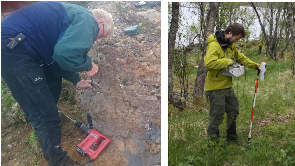
Figure 4.4: Establishing CP ore grounding point and data acquisition in combined CP and SP measurements.
