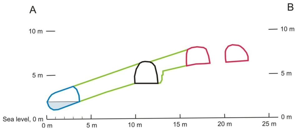
**Figure 53.** Horizontal projection of the Måløy mine together with a vertical section along the western wall of the inclined shaft in the lower part of the figure. Green lines show the location of the inclined shaft connecting the Central adit with the Lower (blue line) and Upper drifts (red line). Stippled lines in the horizontal projection represent underground workings whereas full lines show the location of cuttings at surface.
