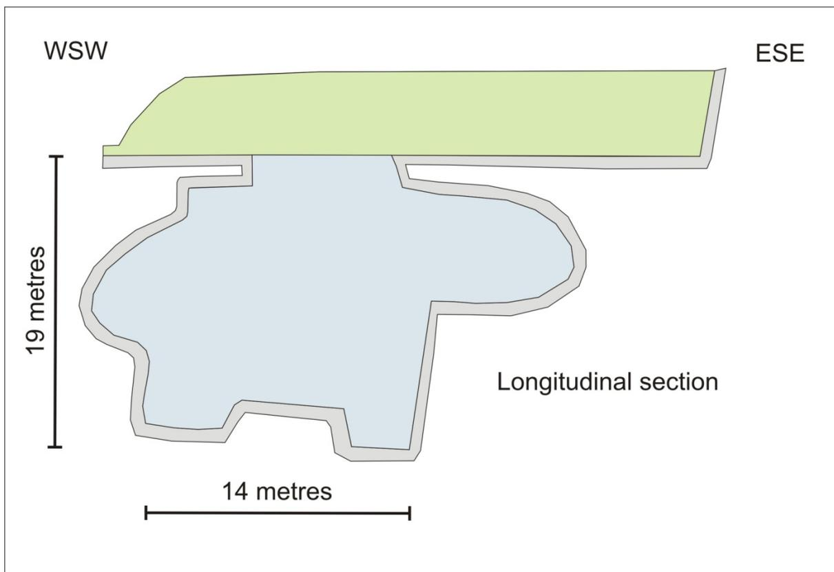
**Figure 45.** Sketch of the longitudinal section of the Lilleålegden mine. The light green area represents the cutting and the light blue area the underground, now water-filled, gallery. Based on the not-to-scale drawing given by Rosenlund and Borthen (1916).
