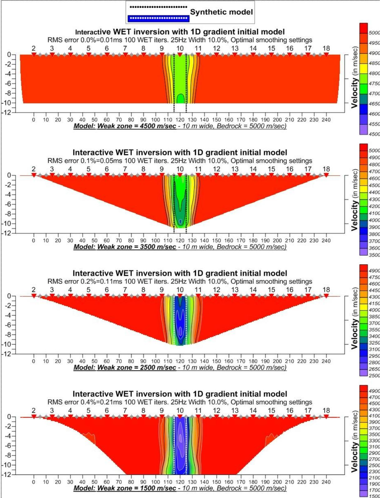
Figure 5.1.1: Effect of velocity contrast between fracture zone and bedrock in single-run WET inversion (weak zone: from top 4500, 3500, 2500 and 1500 m/s).
