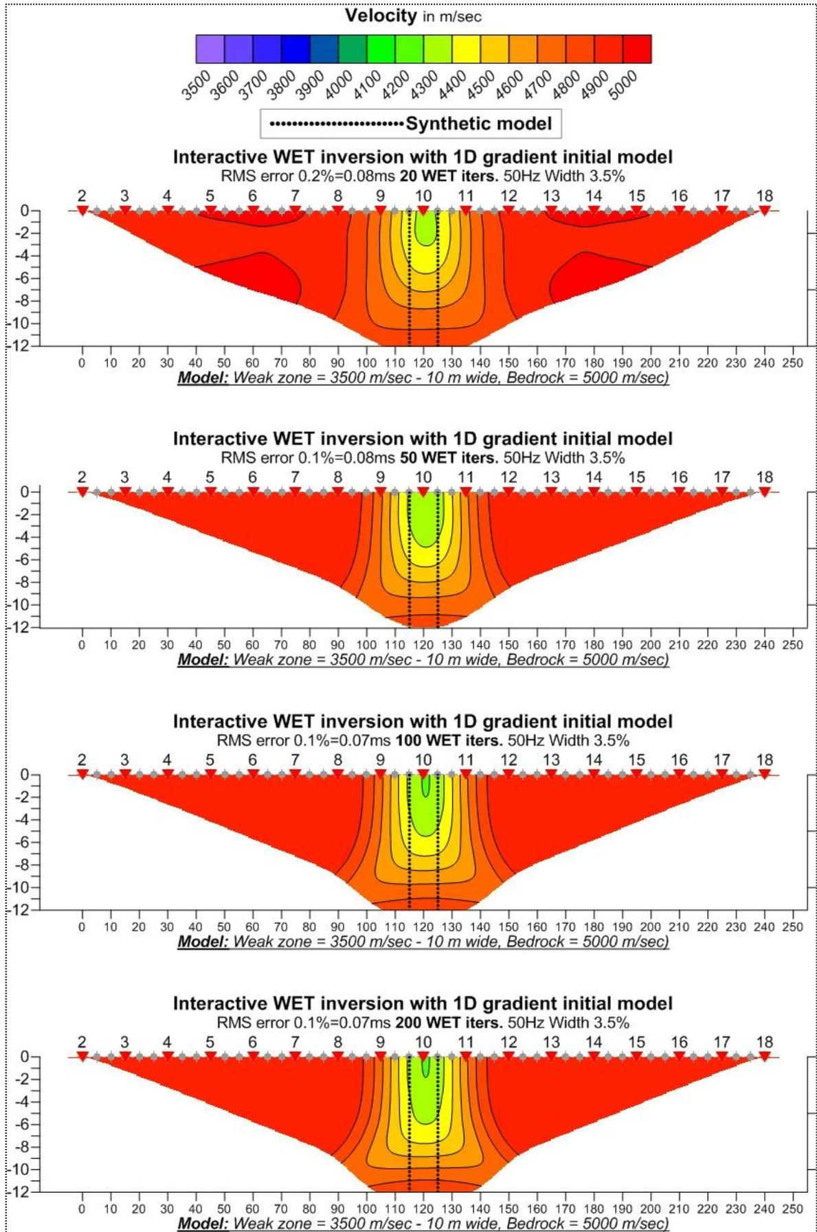
**Figure 4.1:** Effect of number of iterations in single-run WET inversion (from top 20, 50, 100 and 200 iteration test).
