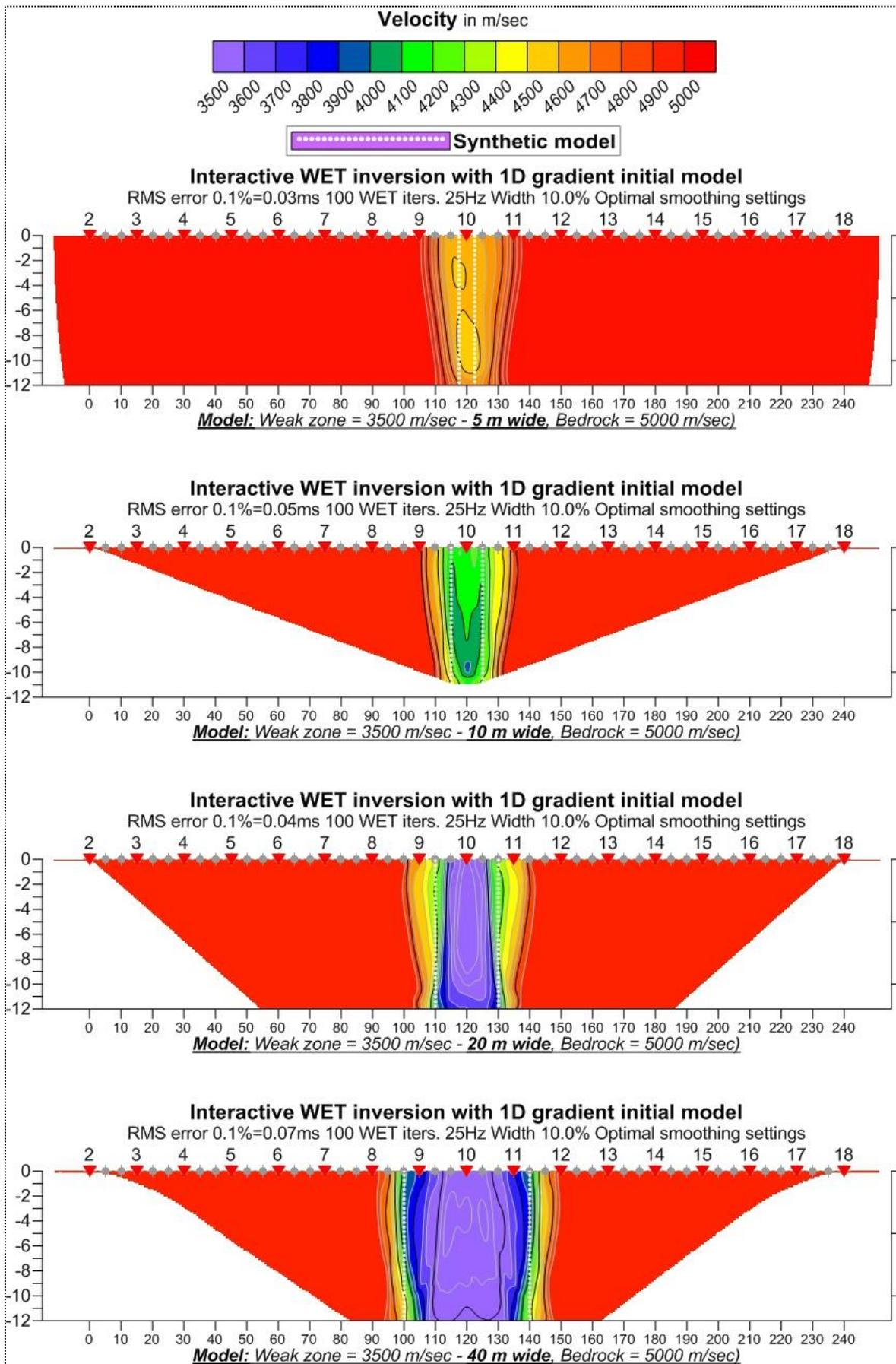
Figure 5.2.1: Effect of fracture zone width in single-run WET inversion (from top 5, 10, 20 and 40 m).
