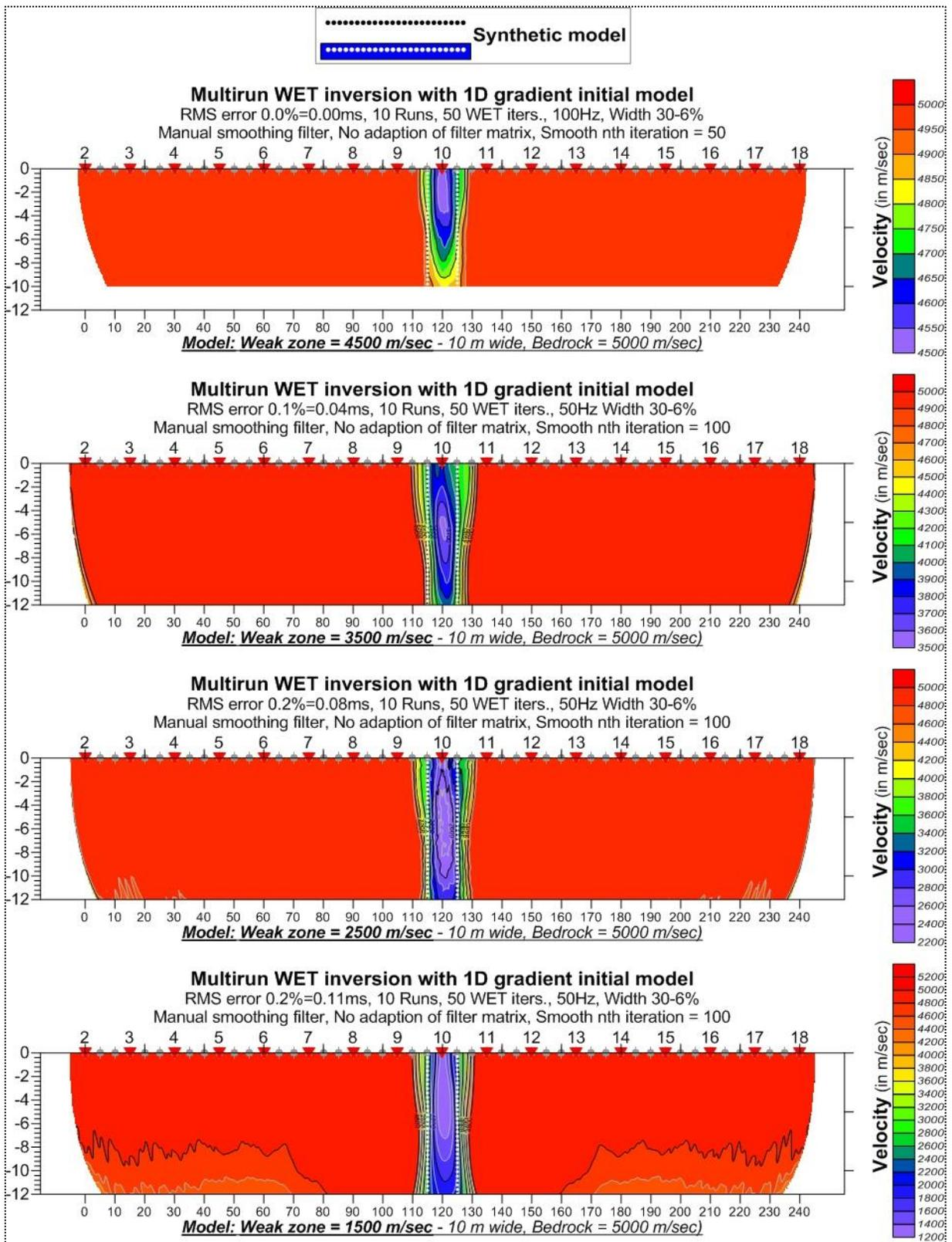
**Figure 5.1.2: Effect of velocity contrast between fracture zone and bedrock in multi-run WET inversion (weak zone: from top 1500, 2500, 3500 and 4500 m/s).**
