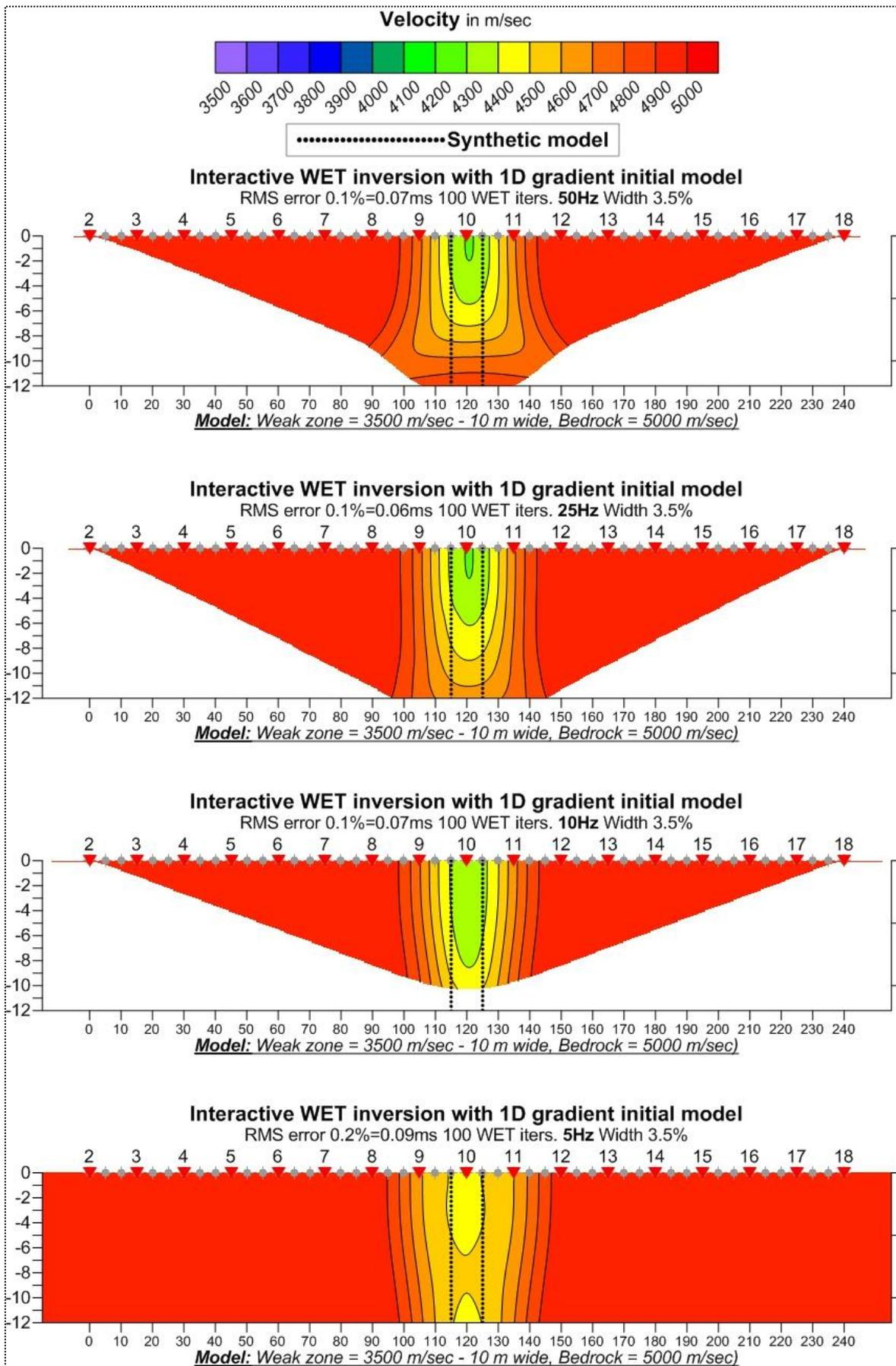
**Figure 4.2:** Effect of decreasing the Wavelength frequency in single-run WET inversion (from top 50, 25, 10 and 5 Hz).
