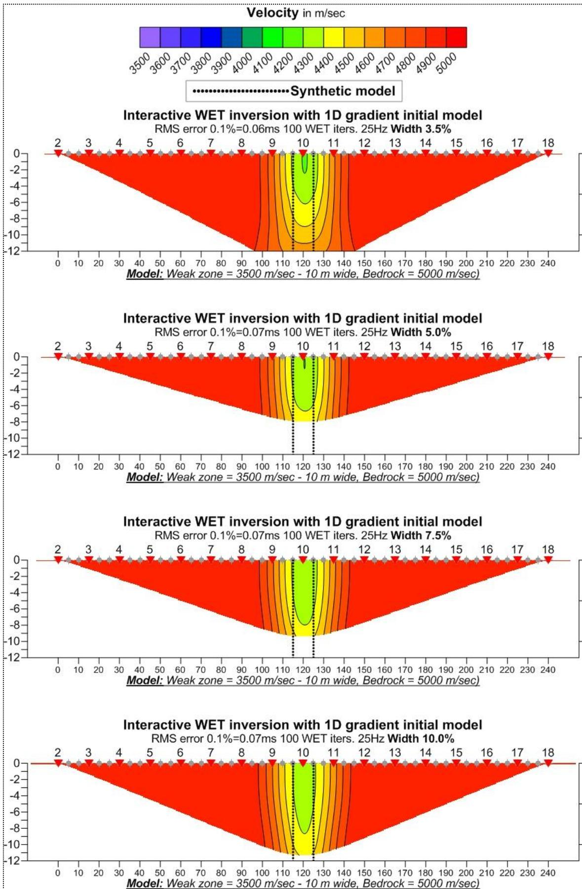
**Figure 4.3:** Effect of increasing the Wavepath width in single-run WET inversion (from top, 3.5, 5, 7.5 and 10%).
