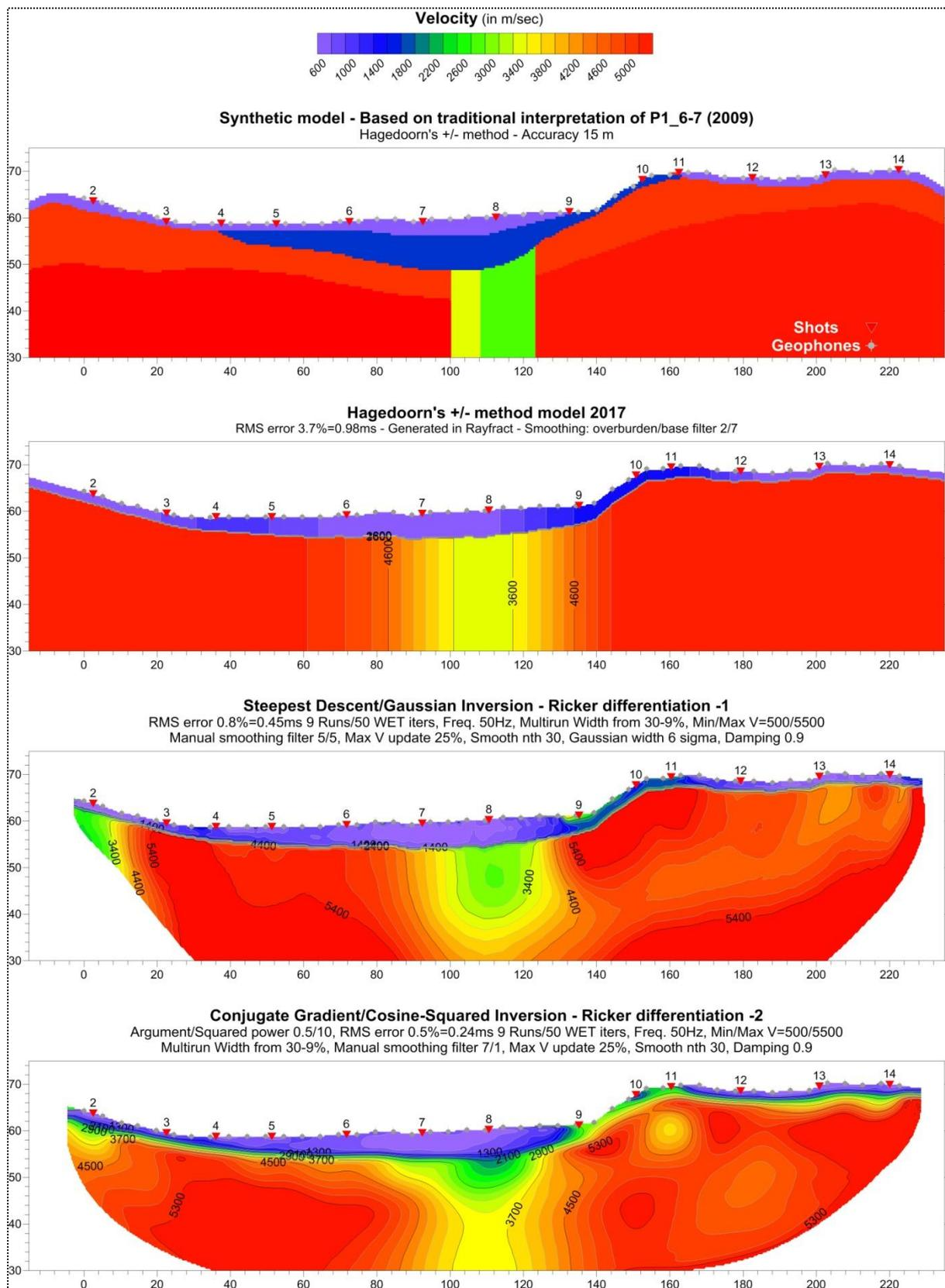
**Figure 6.1.1:** Inversion of synthetic data from a complex model. From top to bottom: synthetic model based on Profile P1\_6-7 from Knappe - 2D Plus-Minus method model as constructed in Rayfract® - Inversion result using the Steepest Descent/Gaussian inversion scheme - Inversion result using the Conjugate Gradient/Cosine-Squared inversion scheme.
