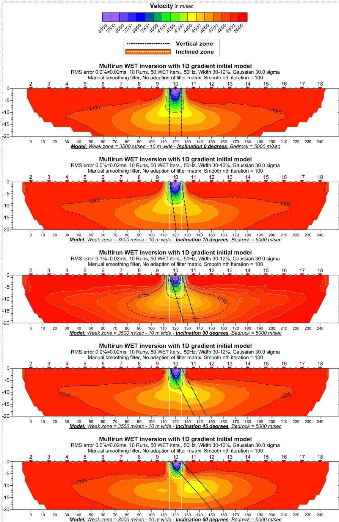
**Figure 5.4.1: Effect of fracture zone inclination in multi-run WET inversion using Conjugate Gradient method and Gaussian weighting (from top 0°, 15°, 30°, 45° and 60° from vertical).**
