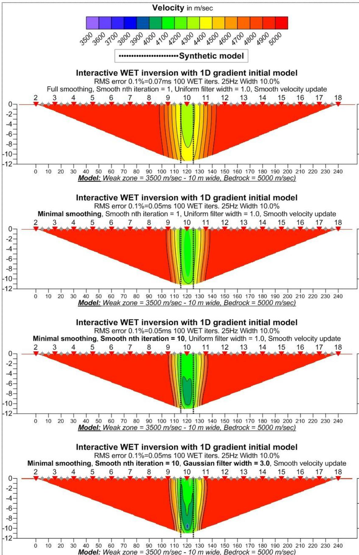
**Figure 4.4:** Effect of editing velocity smoothing prior to single-run WET inversion. Different smoothing parameters are given in the figures headline.
