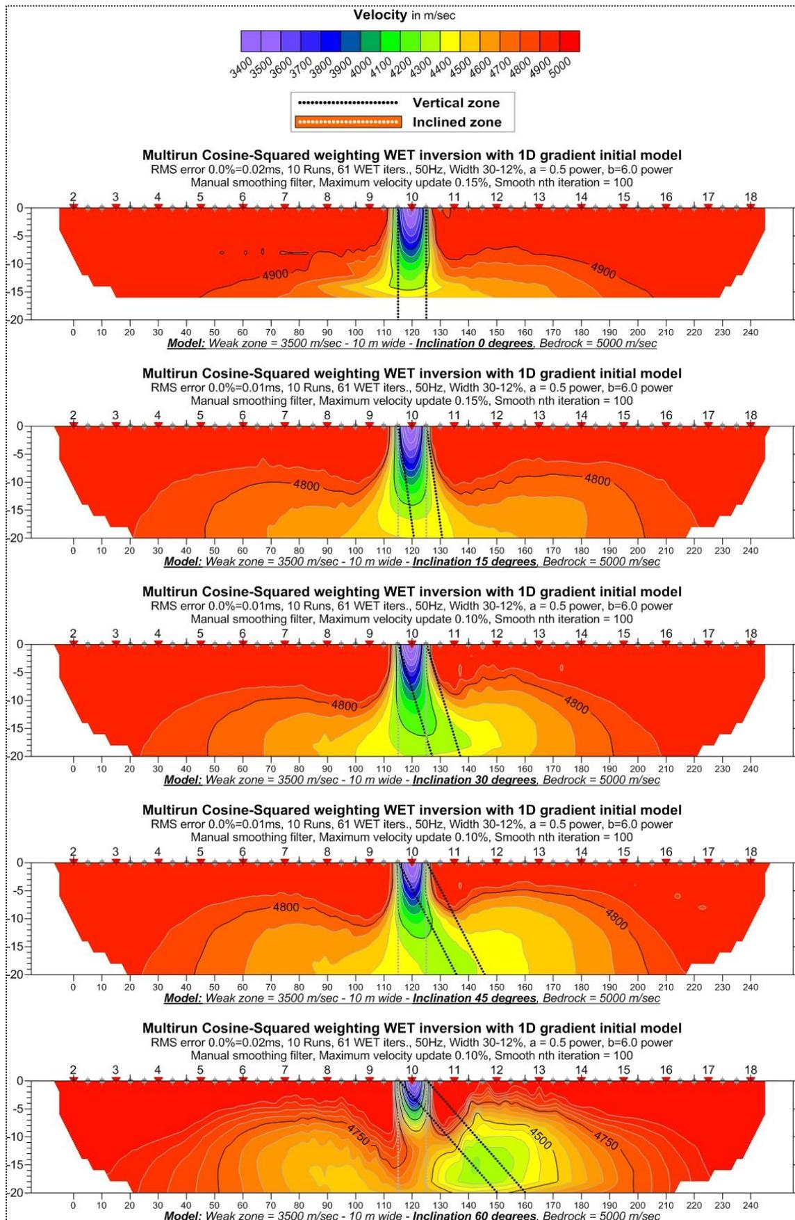
**Figure 5.4.2: Effect of fracture zone inclination in multi-run WET inversion using Conjugate Gradient method and Cosine-Squared weighting ( from top 0°, 15°, 30°, 45° and 60° from vertical).**
