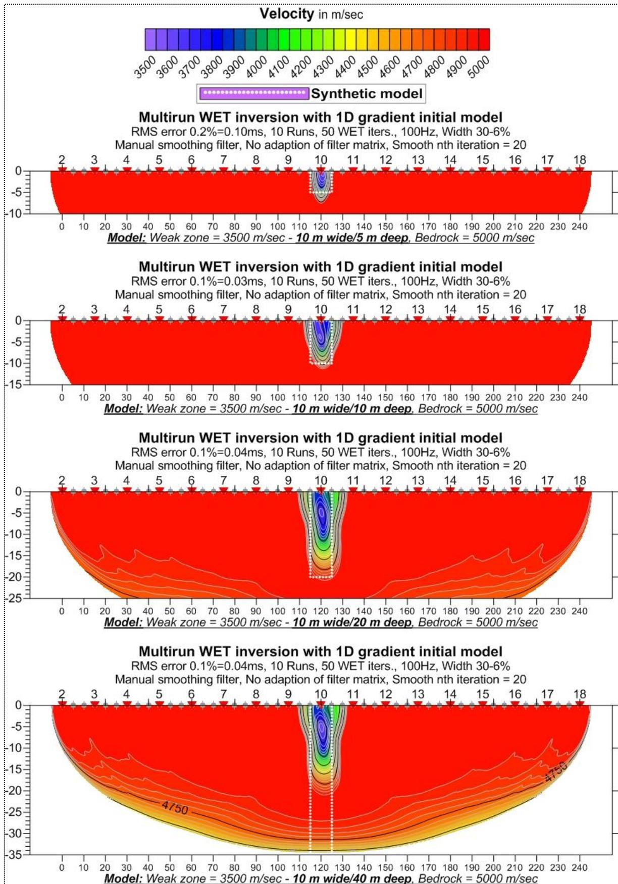
**Figure 5.3.1:** Effect of fracture zone depth in multi-run WET inversion (from top 5, 10, 20 and 40 m).
