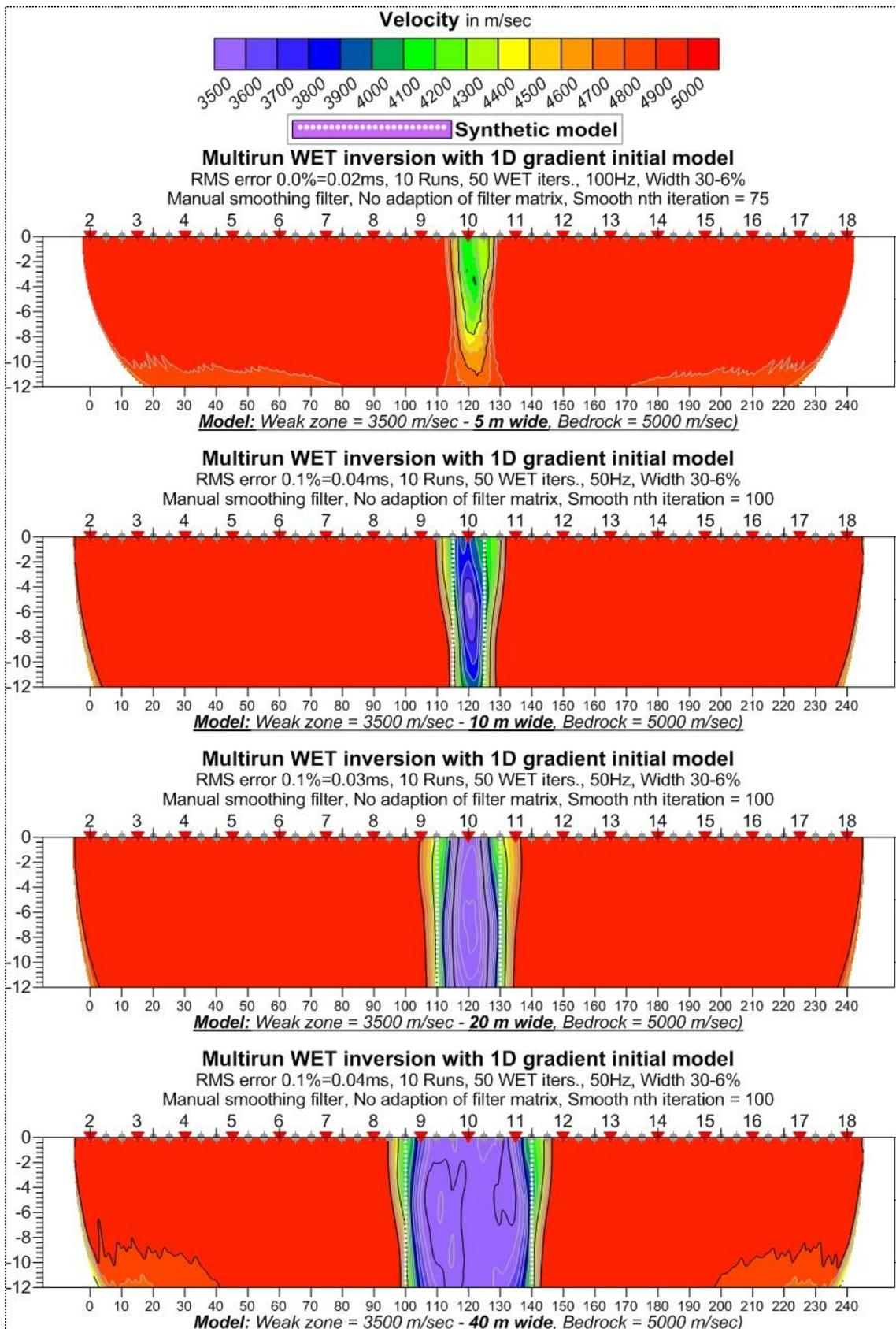
Figure 5.2.2: Effect of fracture zone width in multi-run WET inversion (from top 5, 10, 20 and 40 m).
