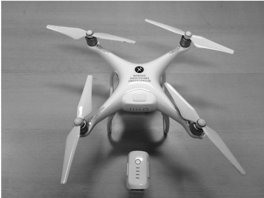
Figure 4.6: The drone used to acquire GPS-rectified images from the air- the DJI Phantom 4.
