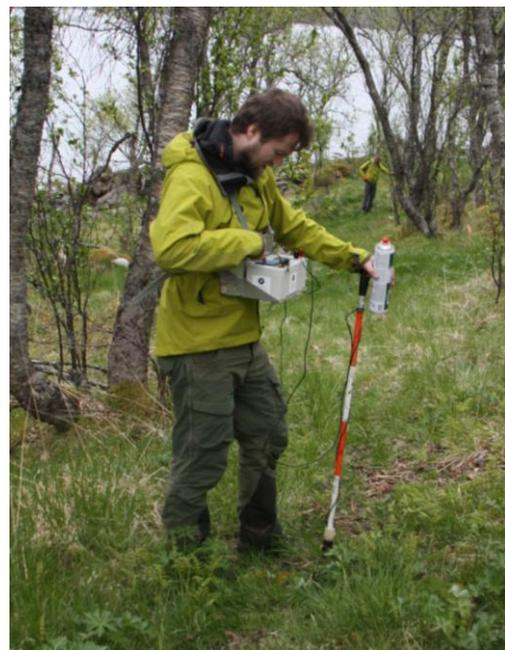
Figure 4.3: Establishing CP ore grounding point and data acquisition in combined CP and SP measurements.
