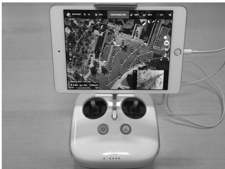
Figure 4.7: The control unit for the DJI Phantom 4 drone with accompanying Ipad. This is used to remotely control the drone with the *Litchi* application.
