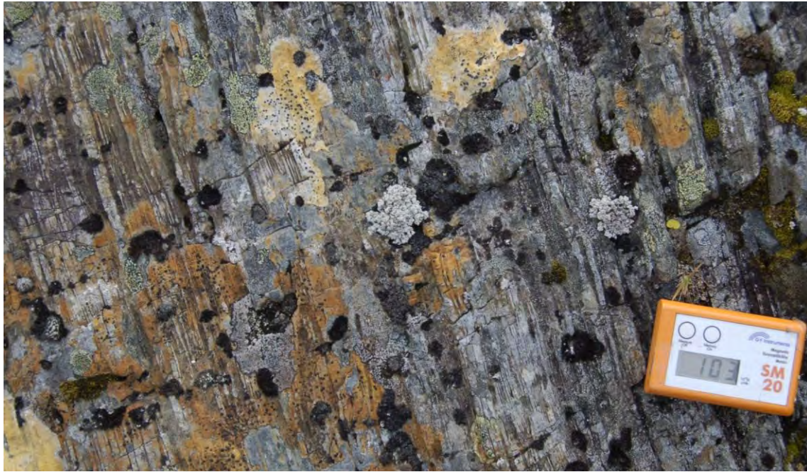
Figure 15: Strongly banded magnetite-rich schist, with alternating quartz-rich and magnetite-rich bands. The susceptibility meter shows a value of 103 \times 10^{-3} SI units, corresponding to c. 3 % magnetite in the rock.
