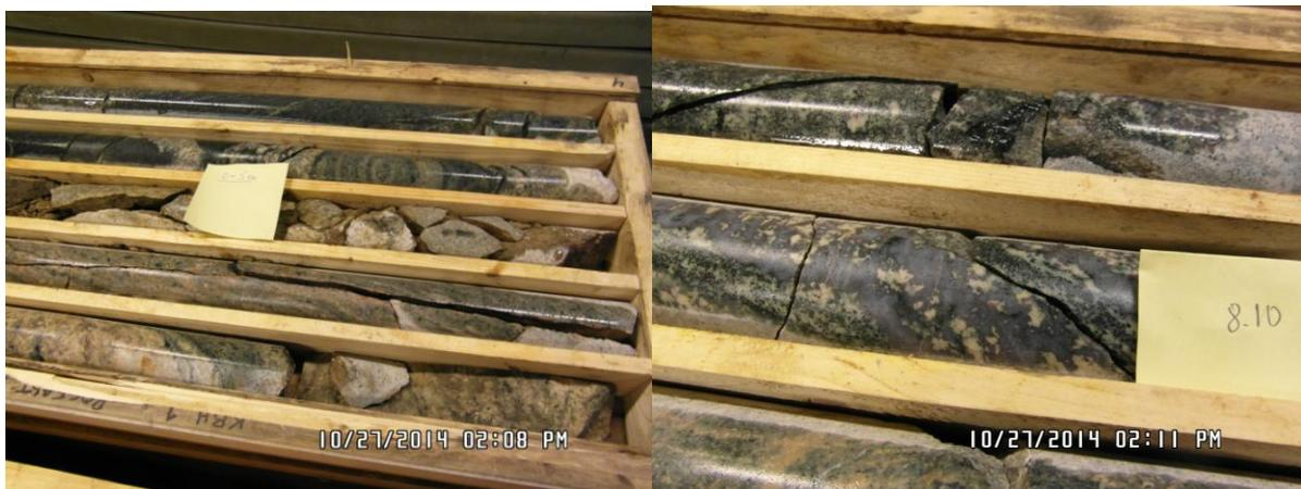
*Fig. 17. A) Core interval between 0-5m that show a lot of fractures. B) Monzonitic(?) gneiss with characteristic blue quartz at core interval c. 8-8.5 m.*
