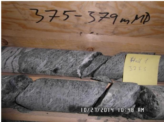
**Fig 4.** Dark schist with characteristic black spots of biotite, Drill core 1, 375-376 m.
