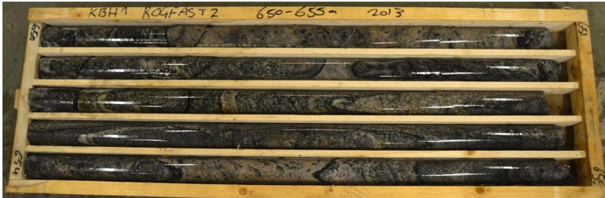
Fig. 25. Relatively leucocratic gneiss of granodioritic composition, core interval 650-655m. Photo by Statens Vegvesen.
