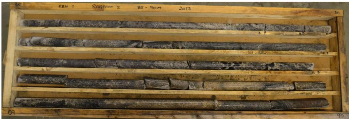
*Fig. 19. Grey gneiss of monzonitic composition at core interval 85- 90 m. Photo by Statens Vegvesen.*
