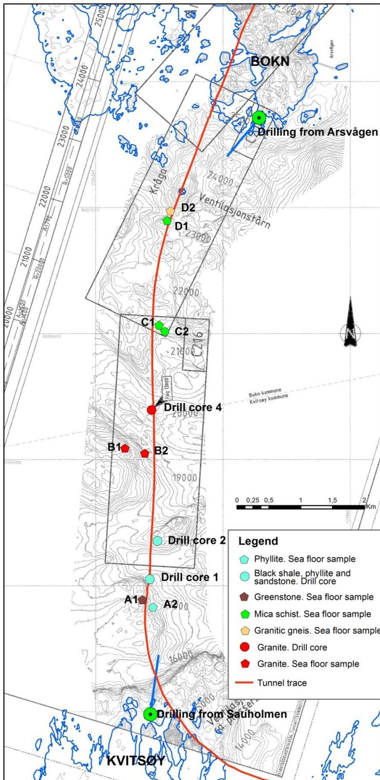
**Fig. 2** Location of drill cores (circles) and seafloor samples (pentagons) in relation to the tunnel trace and drilling from Sauholmen and Arsvågen. The seafloor topography is provided by Statens Vegvesen.
