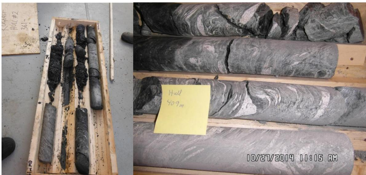
**Fig. 5.** A) Black graphitic shale with only small sections of the core preserved, Drill core 2, 361-367 m. Photo by Statens Vegvesen. B) Grey to green phyllite with lots of quartz veins, but also carbonate bearing. Drill core 2, 409-410 m.
