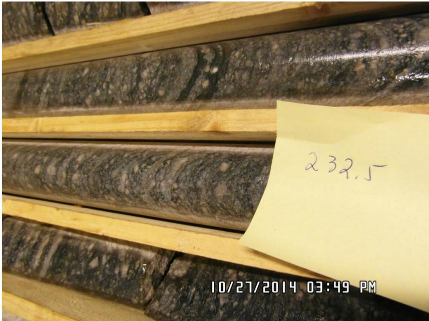
*Fig. 21. Close up of the granitic gneiss with small augens that dominate the core between 210-399 m. The photo it taken at core interval 331-333 m.*
