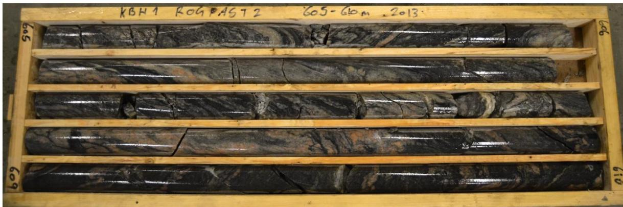
*Fig. 24. Gneiss from the interval 605-610 m. Photo by Statens Vegvesen.*
