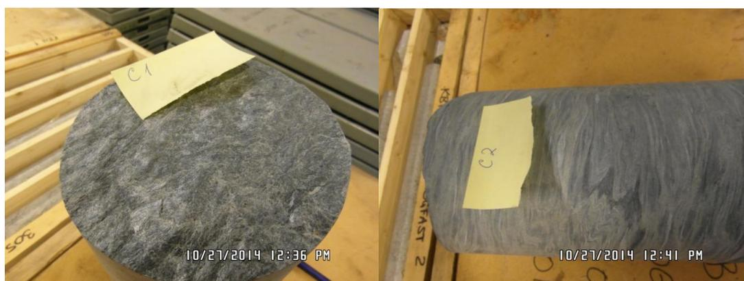
Fig. 9. A) Sample C1, mica schist, sample seen from the end. B) Sample C, phyllite or mica schist, rather quartz rich, with recumbent folds.
