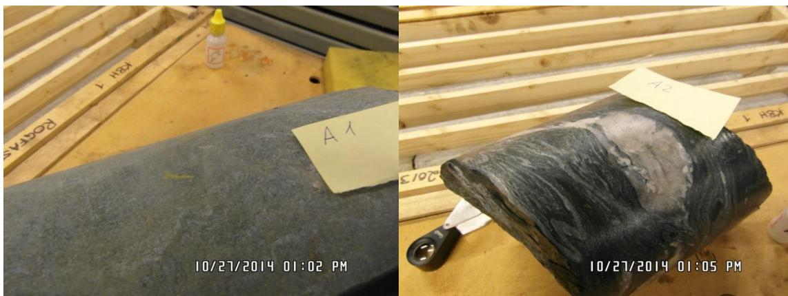
*Fig. 7. A) Sample A1, greenstone. B) Sample A2, green phyllite with a quartz lens and small veins of quartz. Carbonate bearing.*
