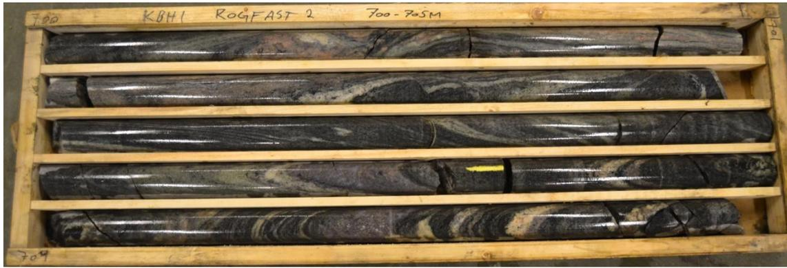
Fig. 12. Arsvågen drill core, interval 700-705 m. Granitic to granodioritic migmatitic gneiss. This is a typical rock type for a major part of the core from Arsvågen. Photo by Statens Vegvesen.
