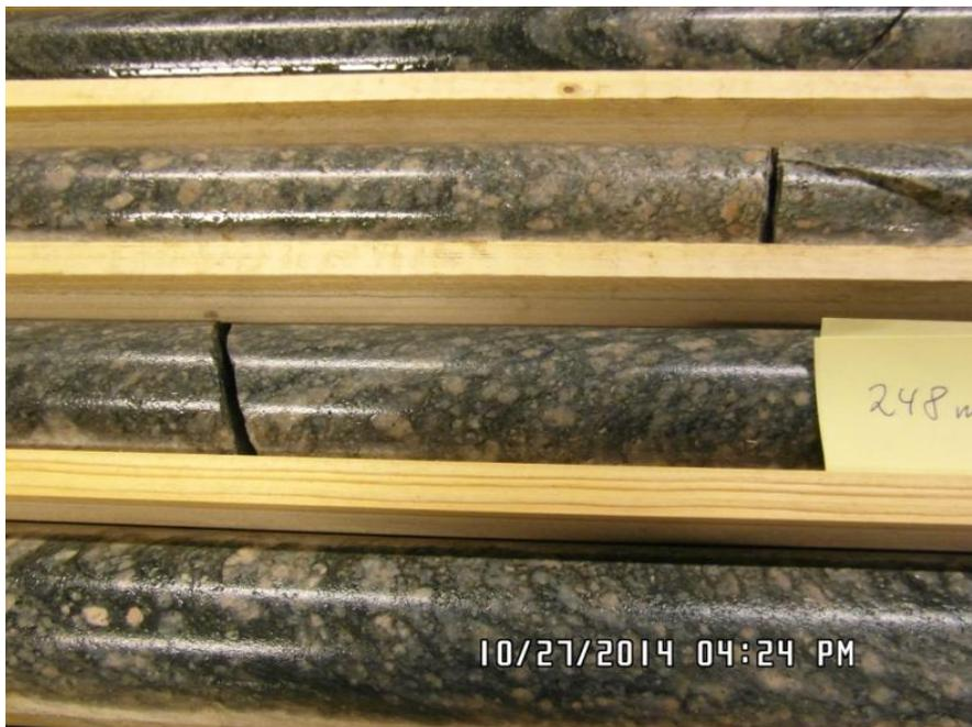
*Fig. 11. Arsvågen drill core at interval 247-249 m. Porphyritic granitic gneiss.*
