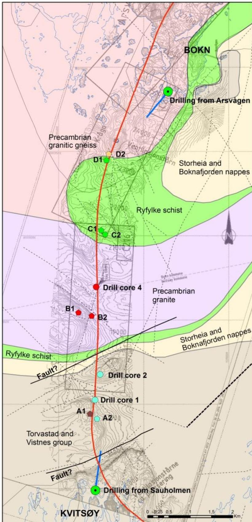
Fig.13 . Detailed geological map along the tunnel trace between Kvitsøy and Bokn. The colors are pale compared to Fig.14 in order to show the seafloor topography. The stippled line are lineaments taken from earlier reports. Some possible faults are indicated. See legend in Fig.2 for explanation of drill cores (circles) and seafloor samples (pentagons).
