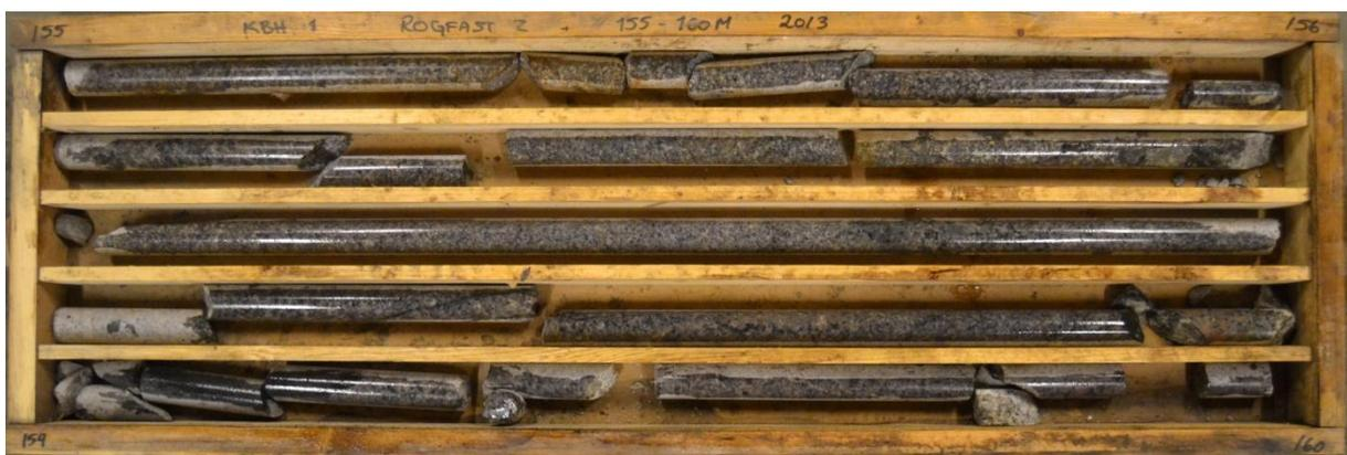
*Fig. 20. Monzonite or monzonitic gneiss, only weakly foliated. Core interval 155-160 m. Photo by Statens Vegvesen.*
