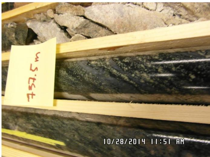
Fig 27. Close-up of migmatitic gneiss with blue quartz at core interval c. 737.5m.
