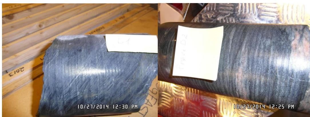
Fig. 10A) Sample D1. Phyllite or mica schist. B) Sample D2. Strongly foliated migmatitic granitic gneiss.
