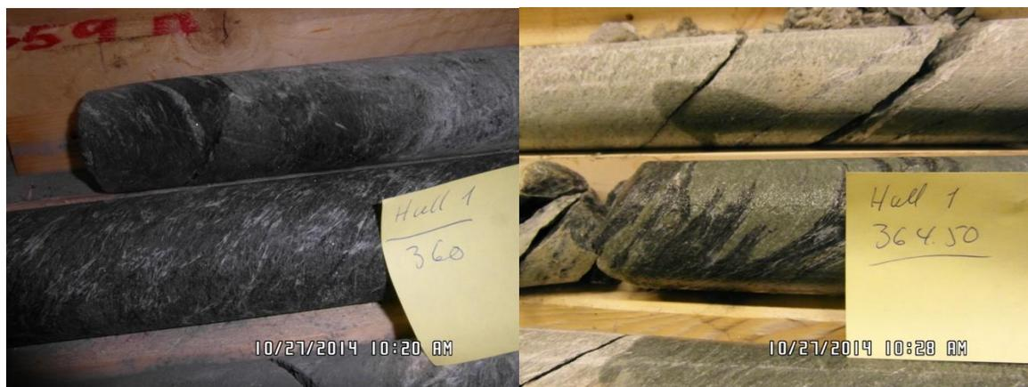
*Fig. 3. A) Dark shale with carbonate veins from Drill core 1 at 360m. B) Sandstone with black shale interfingering, Drill core 1 at 364.5m*
