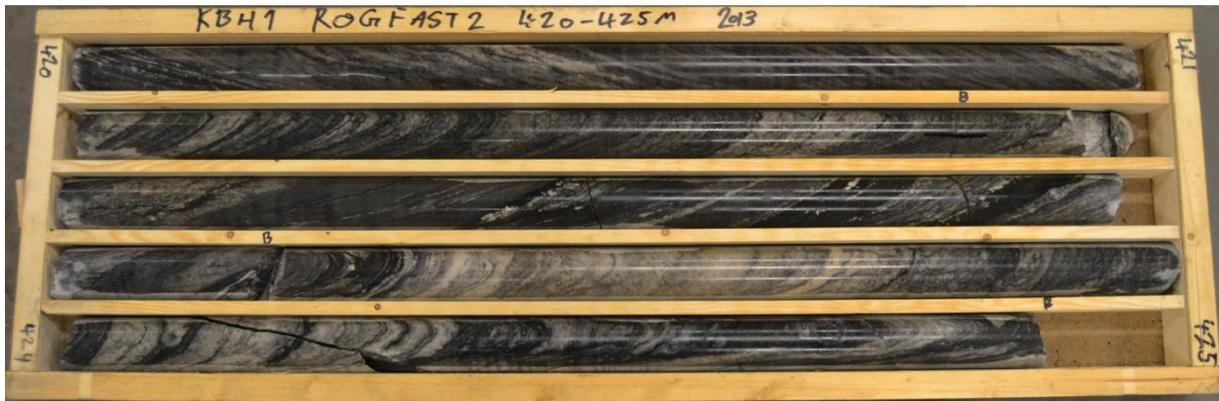
*Fig. 23. Typical grey granitic or granodioritic gneiss that dominates the lower half of the core from Arsvågen. Here at interval 420-425. Photo by Statens Vegvesen.*
