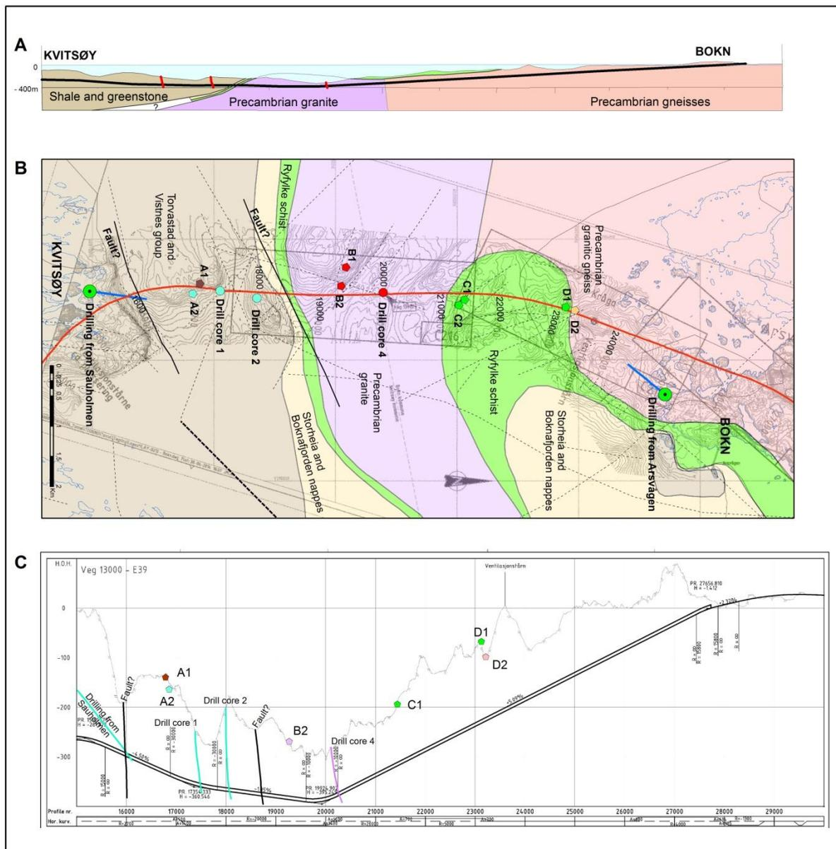
Fig. 15. A) Section along the tunnel trace nearly at the correct proportions. The tunnel trace is shown as a thick black line, and the drilled cores as short red lines. B) Detailed geology along the tunnel as shown in Fig 13. C) Seafloor samples and drill cores along the tunnel profile. The vertical axis is about ten times exaggerated. The drilling from Sauholmen is indicated. Topography provided by Statens Vegvesen. The three sections are not quite to scale.
