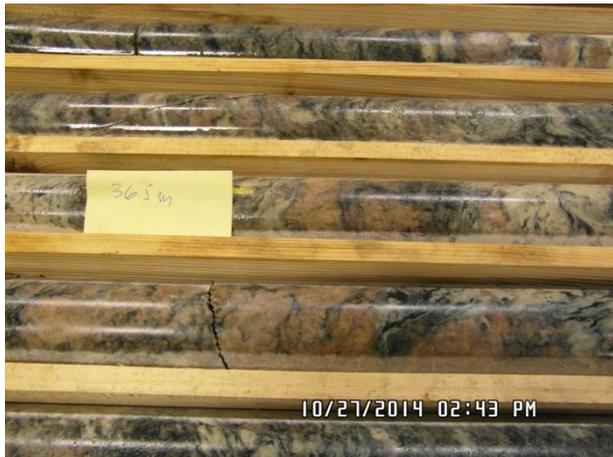
*Fig 18. Red, rather coarse grained gneiss, core interval c. 36.5-37.5m*
