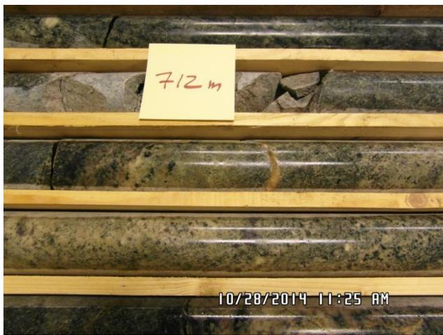
Fig 26. Weakly foliated tonalite with a greenish color, core interval c. 712-713 m.
