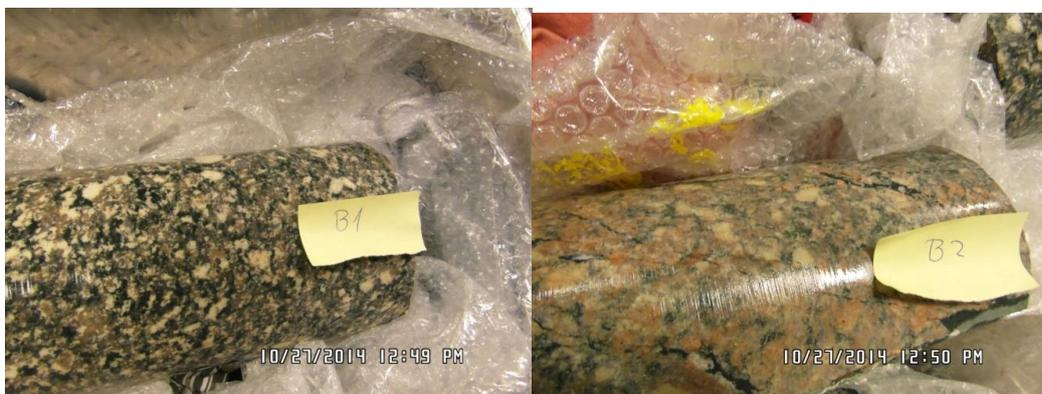
*Fig. 8. A) Sample B1, granite. B) Sample B2, red granite with joints filled with chlorite.*
