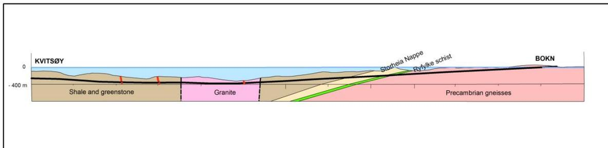
Fig. 16. Alternative section, (cf. Fig. 15 A) where the granite in the central part of the tunnel is interpreted as part of the Vest-Karmøy Suite and separated by fault from the Torvastad Group. Other symbols as in Fig. 15A.
