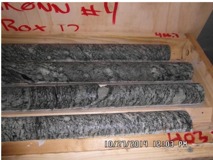
*Fig. 6. Porphyritic granite with continuous core, Drill core 4, 400-403 m. The main part of the drill core looks like this.*
