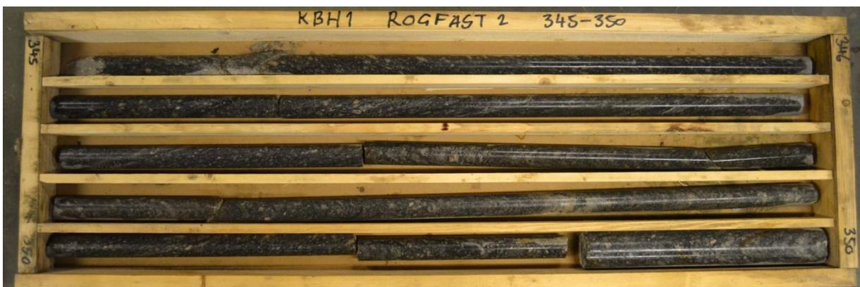
*Fig 22. Core interval 345-350 m that shows the granitic gneiss with small augens and very coherent cores. Photo by Statens Vegvesen.*
