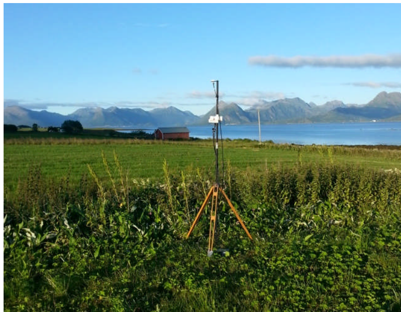
Figure 3: A GEM GSM-19 magnetic base station.
