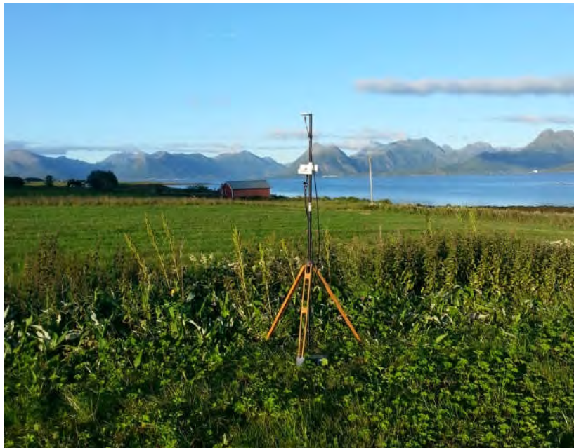
Figure 3: A base station magnetometer (GEM GSM-19) installed 8.5 km southwest of Sortland
