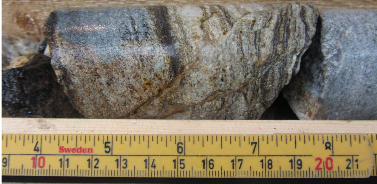
Figure 20. Old fault at 72.10 to 72.20 meter showing displacement along sealed fractures and appurtenant fault rock such as cataclasite; cohesive and cemented fault rock.
