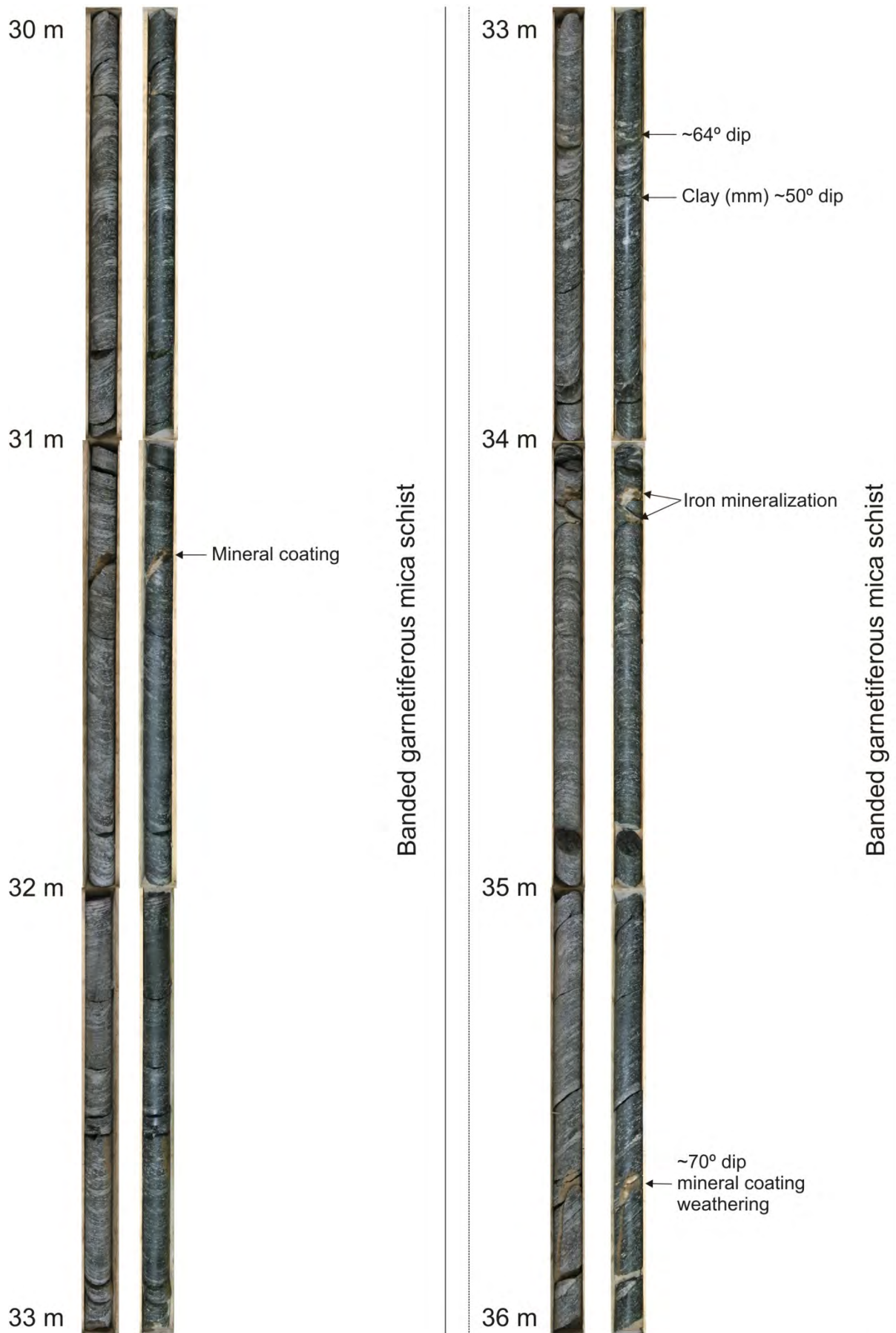
Figure 30. Core logging of drill core BH 02-13 at 30-36 m. Photo of dry core to the left and wet core to the right.
