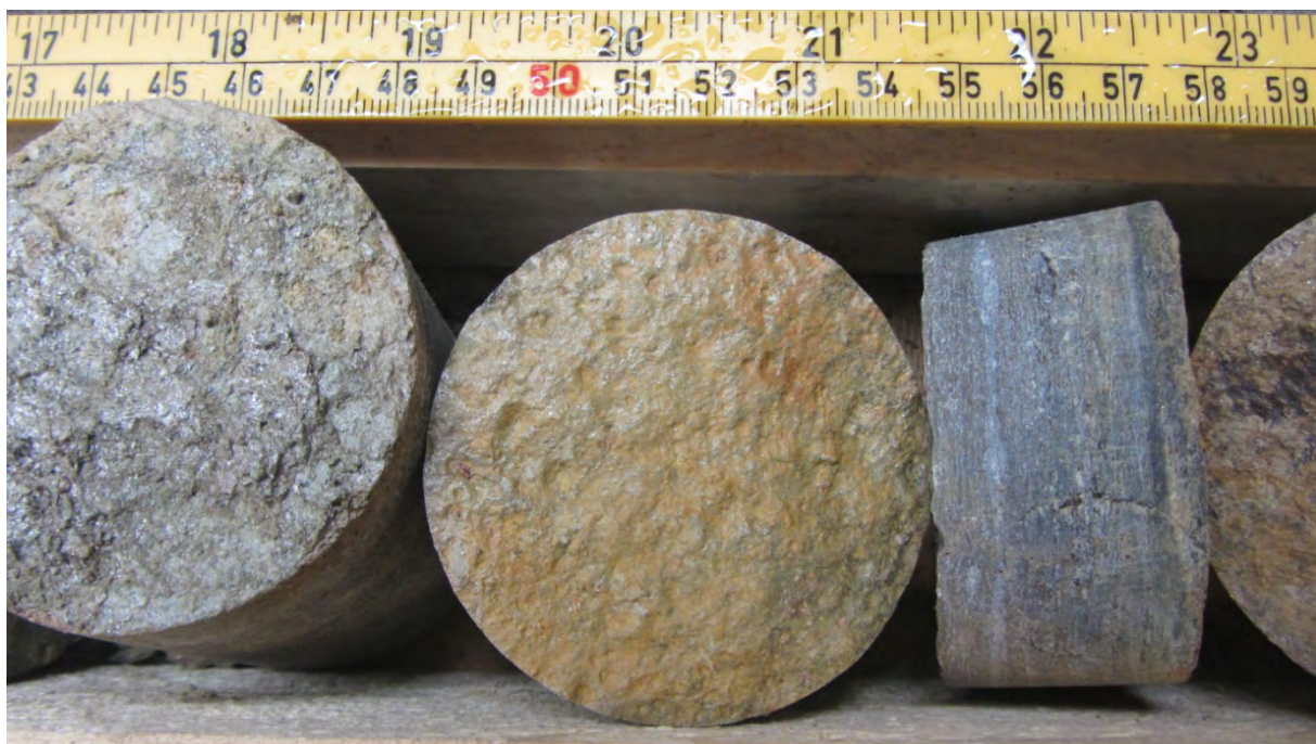
Figure 15. Example of iron oxidation (middle) and clay (mica) coating (left) on fractures. Here at ca. 23.50 m.
