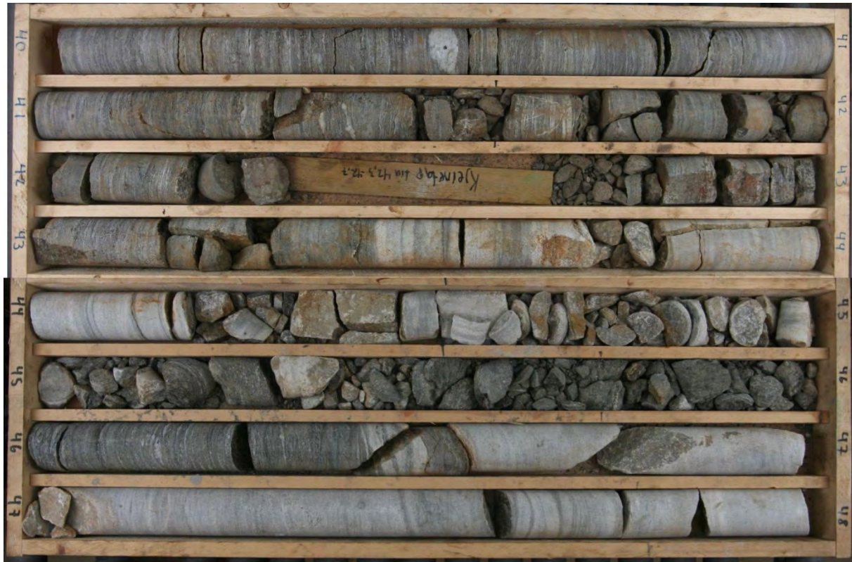
Figure 18. Main zone in BH 3 at 42.3 to 46 meter. The beginning of this zone is lost due to core loss, where the rest of the 3.7 m wide zone is dominated by crushed rock. The bedrock alters between mica schist to marble from top to bottom.
