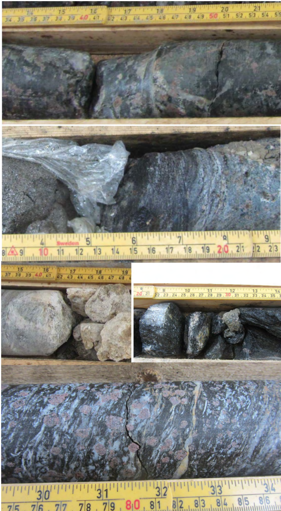
Figure 3. Examples of fractures produced by the drilling process. Top two photos; slimming of drill core. Mid left; rounded edge of drill core. Bottom; irregular fracture.
