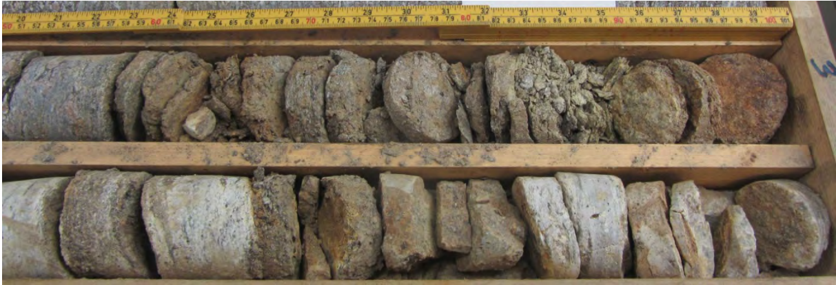
Figure 5. Photo shows an example from the upper 2.5-4 m where the mica rich schist is heavily fractured, weathered and oxidized.
