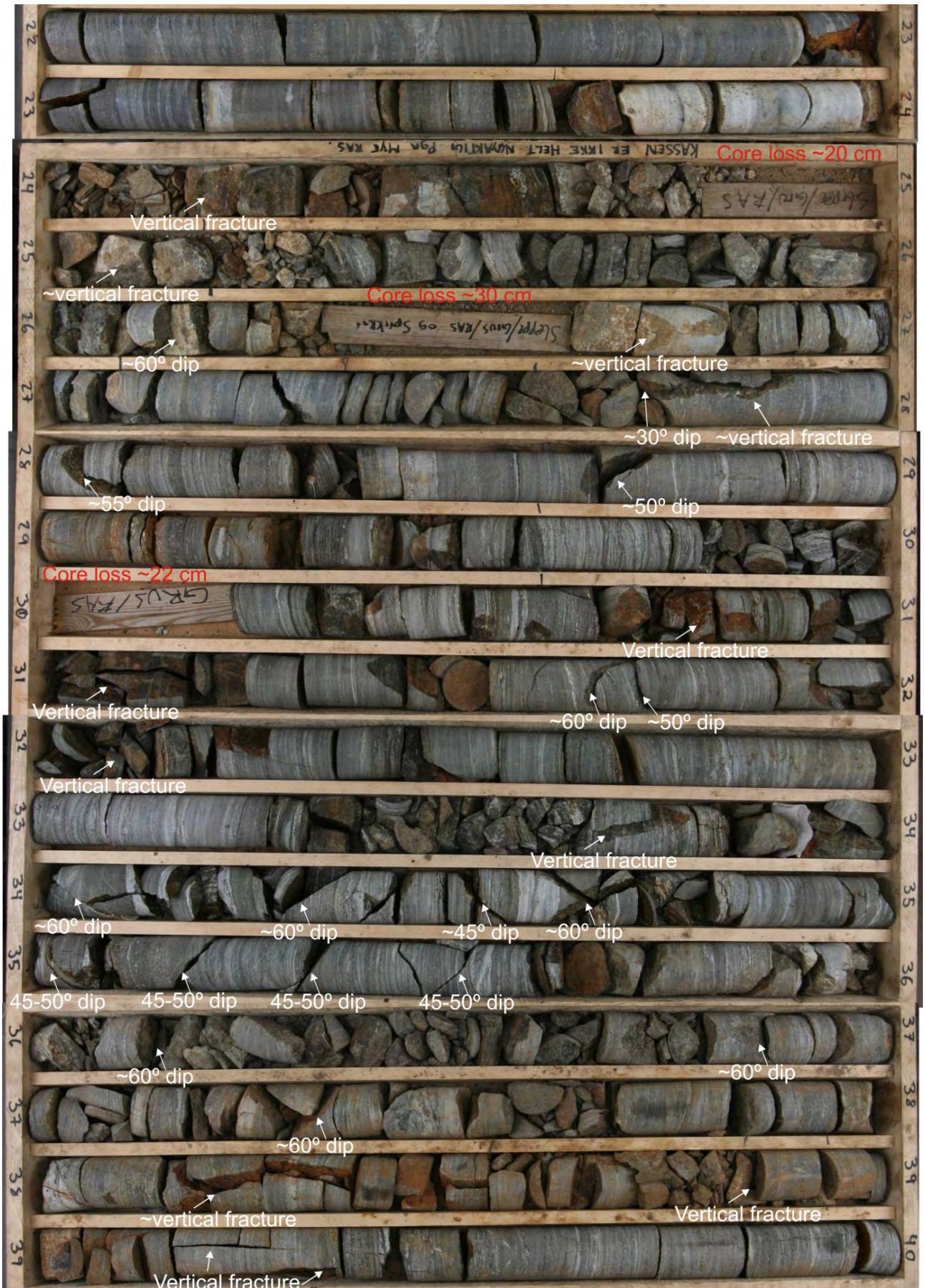
Figure 16. Zone of crushed rock from ca. 24 to ca. 36.80 m where the bedrock is crushed and core loss occurred. Core segment is 1 m.
