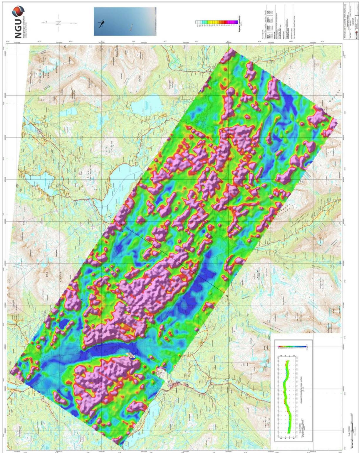
Figure 9. Apparent resistivity. Frequency 880 Hz, Coplanar coils
