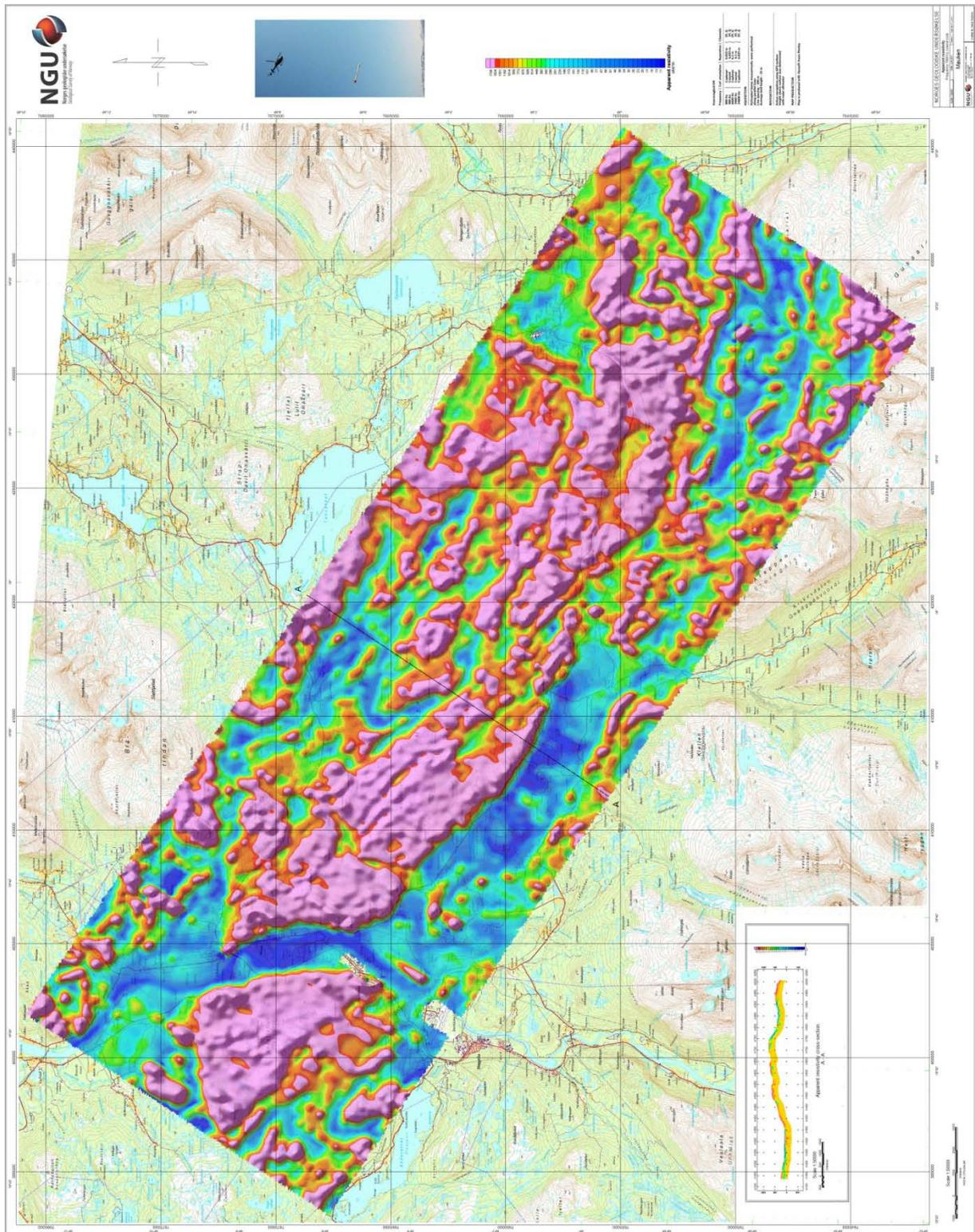
Figure 10. Apparent resistivity. Frequency 7000 Hz, Coaxial coils
