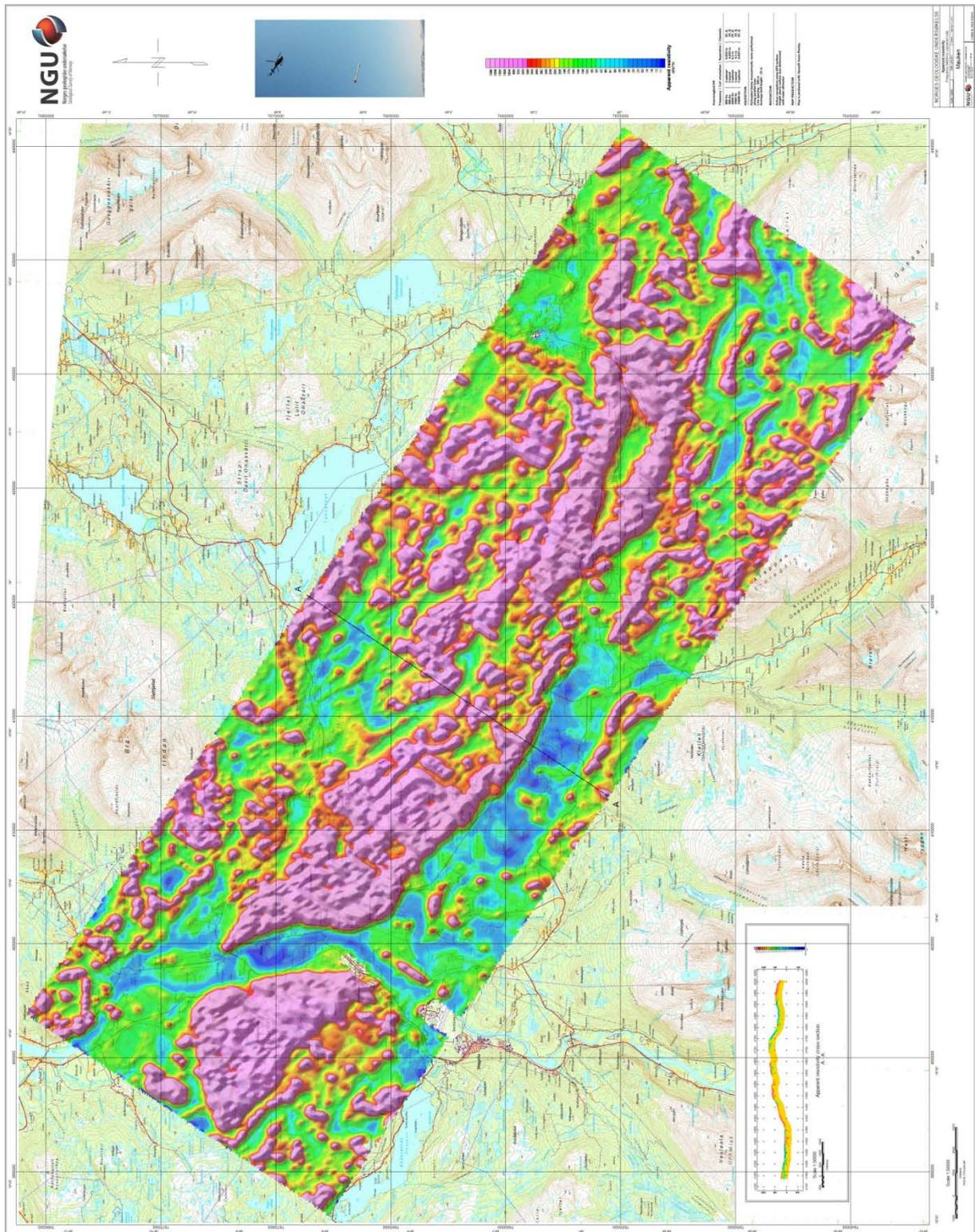
Figure 7. Apparent resistivity. Frequency 3400 Hz, Coplanar coils
