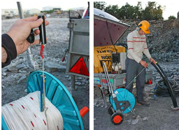
**Fig. 2.2:** VEMCO minilogger and sinker bound to a chord with two meter marks for manual depth determination (left) and temperature logging inside the collector pipe (right).
