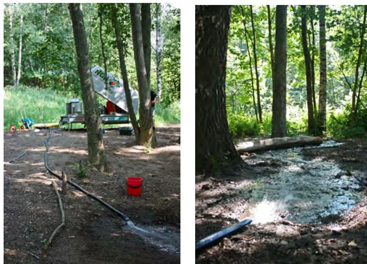
**Fig. 2.8:** TRT setup at borehole 3 for the test with pumping of groundwater and water removal with a fire hose.
